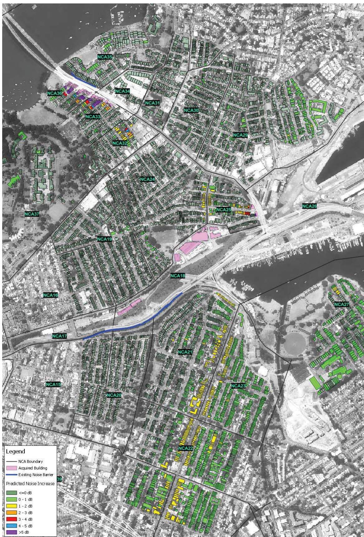
Figure 8-1 Predicted change in noise levels with project without mitigation (daytime – 2033)
