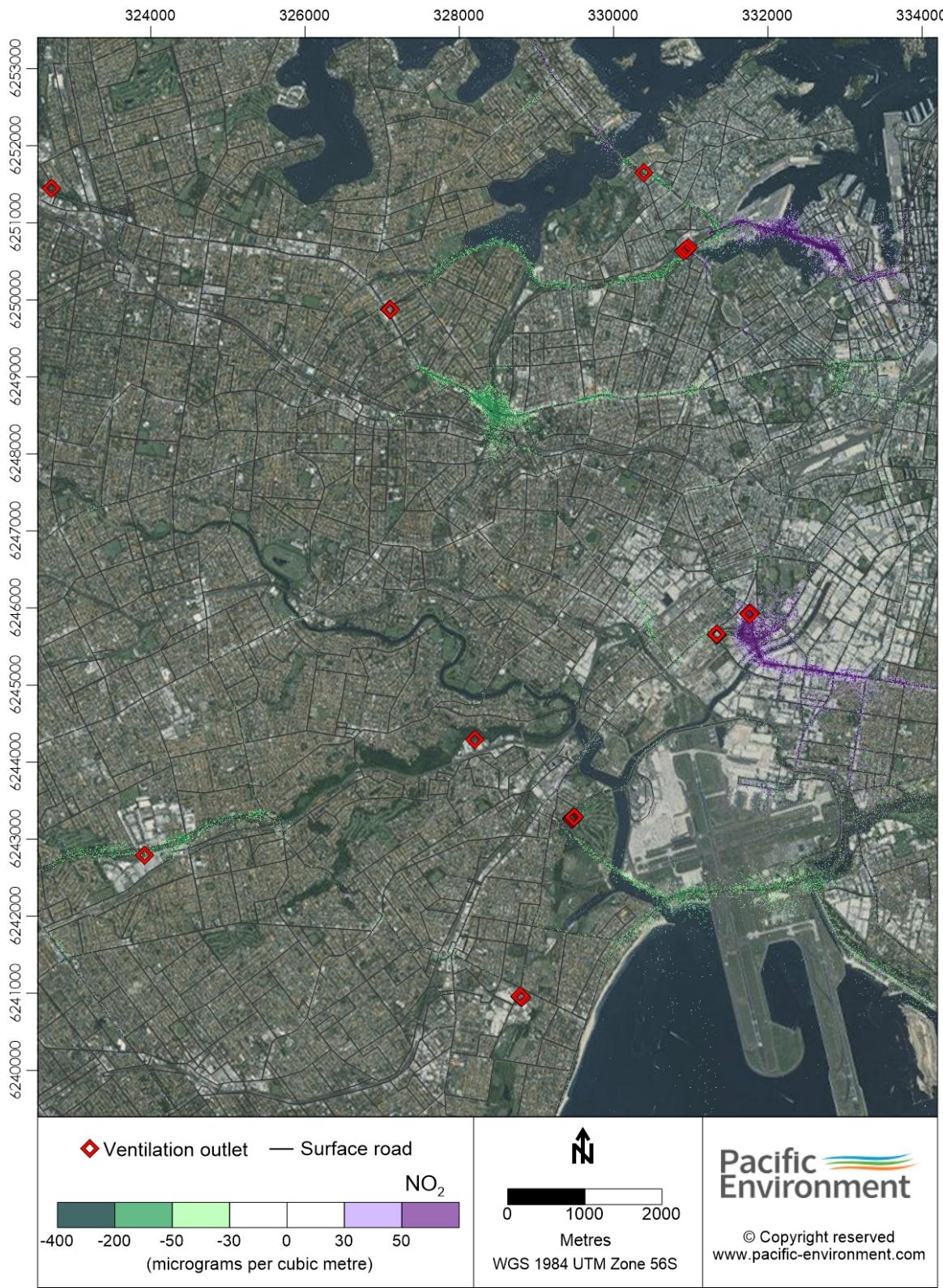
**Figure K-40 Contour plot of change in maximum 1-hour mean  $\text{NO}_2$  concentration in the 2033 Do Something scenario (all sources, 2033-DS minus 2033-DM)**
