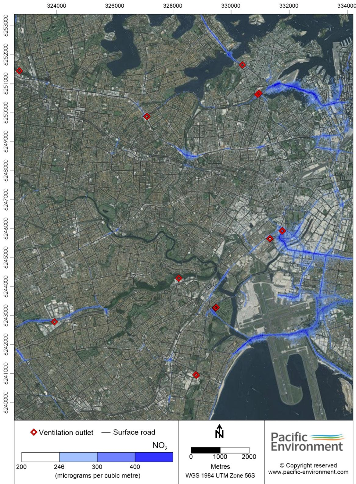
**Figure K-39 Contour plot of maximum 1-hour mean  $\text{NO}_2$  concentration in the 2033 Do Something scenario (all sources, 2033-DS)**
