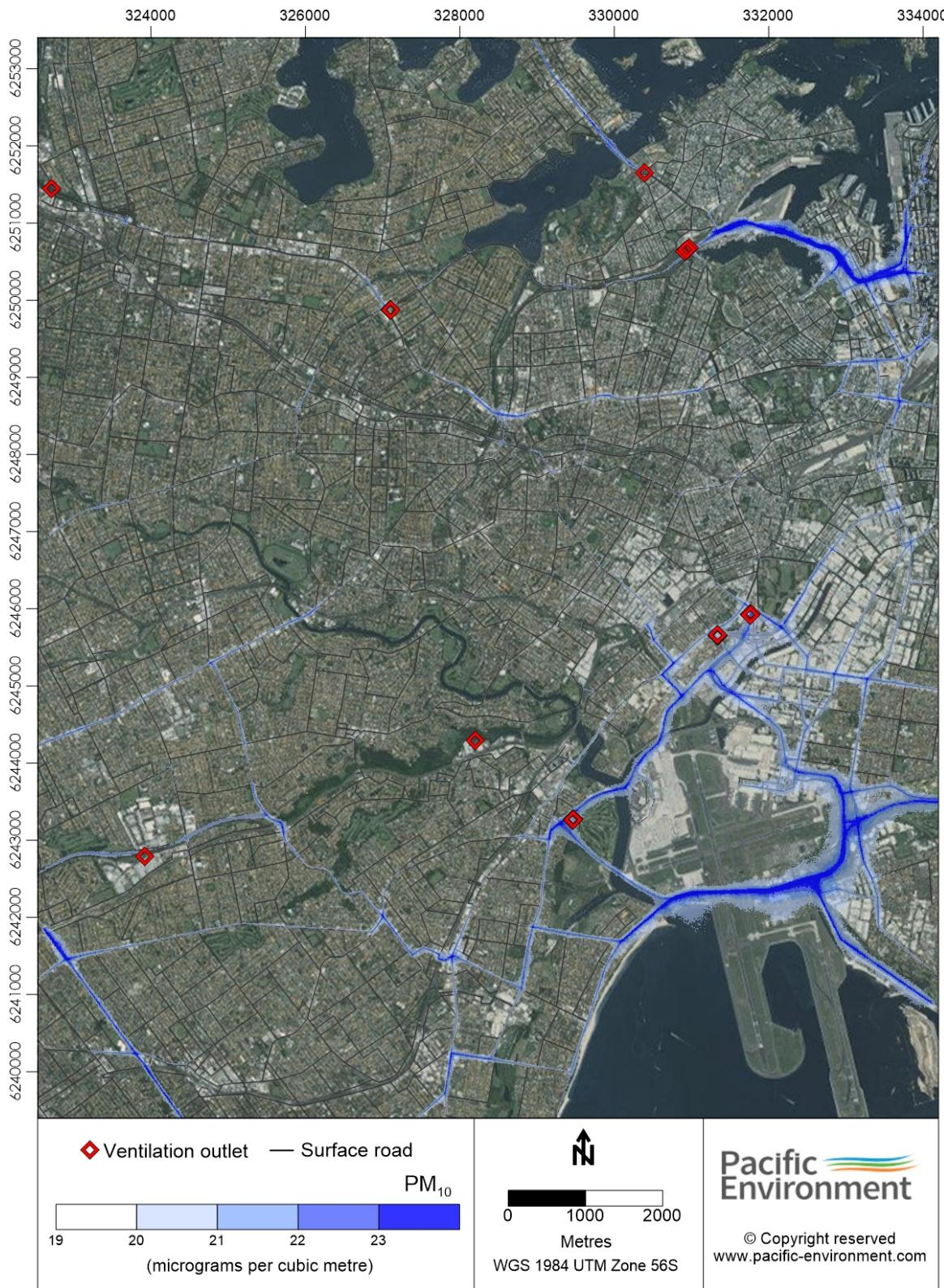
**Figure K-55 Contour plot of annual mean PM<sub>10</sub> concentration in 2023 cumulative scenario (all sources, 2023-DSC)**
