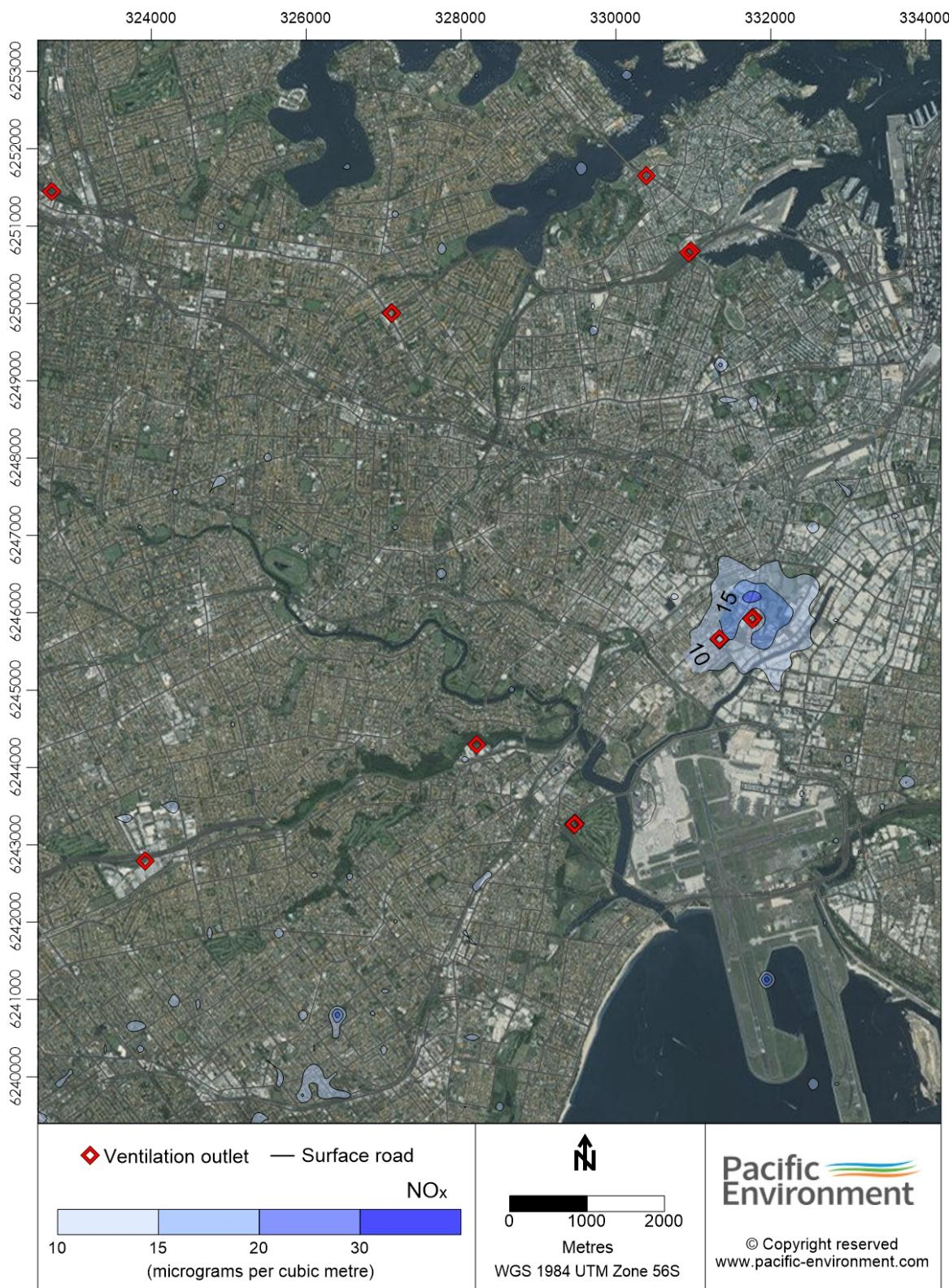
**Figure K-45 Contour plot of maximum 1-hour NO<sub>x</sub> concentrations (ventilation outlets only, 2033-DS)**
