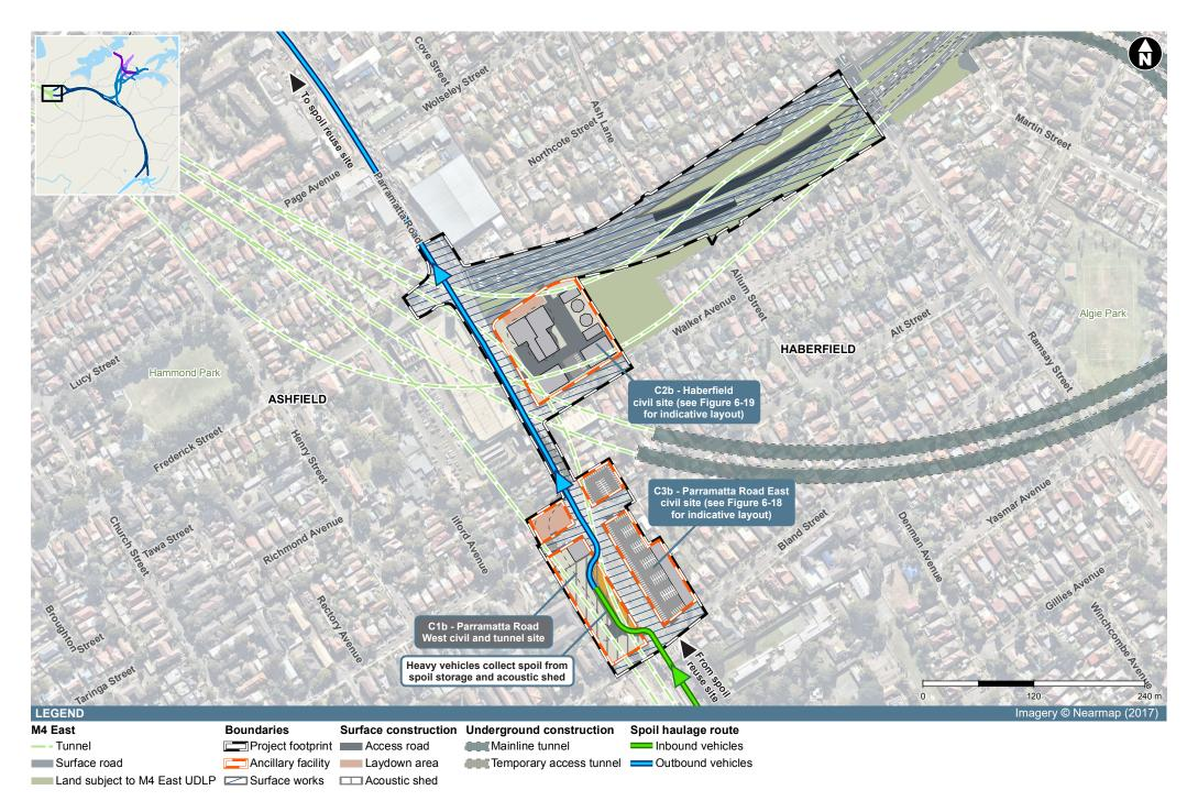
Figure 6-27 Indicative spoil haulage route – Parramatta Road West civil and tunnel site (C1b)
