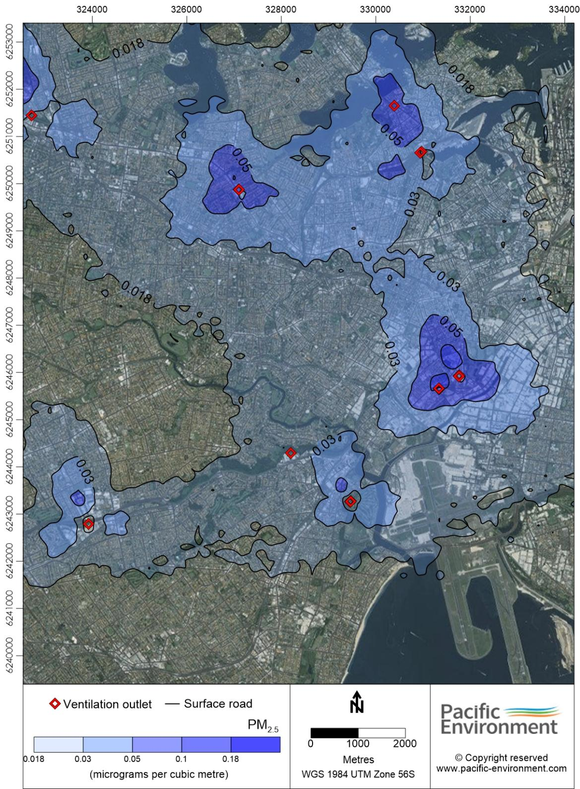
**Figure K-100** Contour plot of annual mean PM<sub>2.5</sub> concentrations (ventilation outlets only, 2023-DS)
