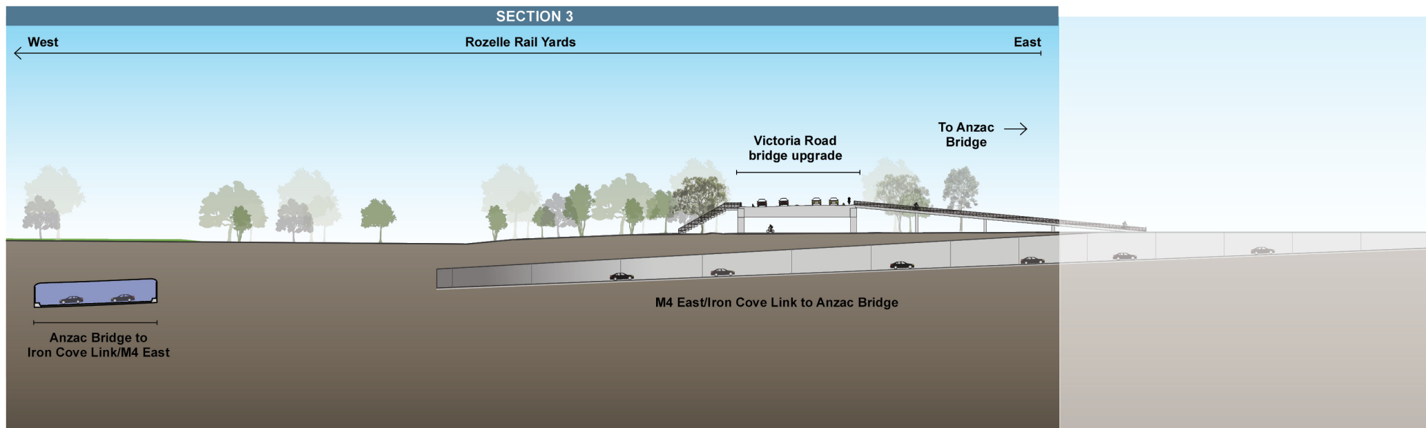
Figure 5-36 Long-section of the Rozelle Rail Yards - east-west - section 3
