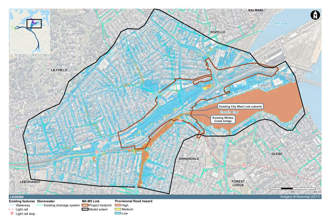
Figure 4-8 Present day flood behaviour – Rozelle interchange - provisional flood hazard (100 year ARI)
