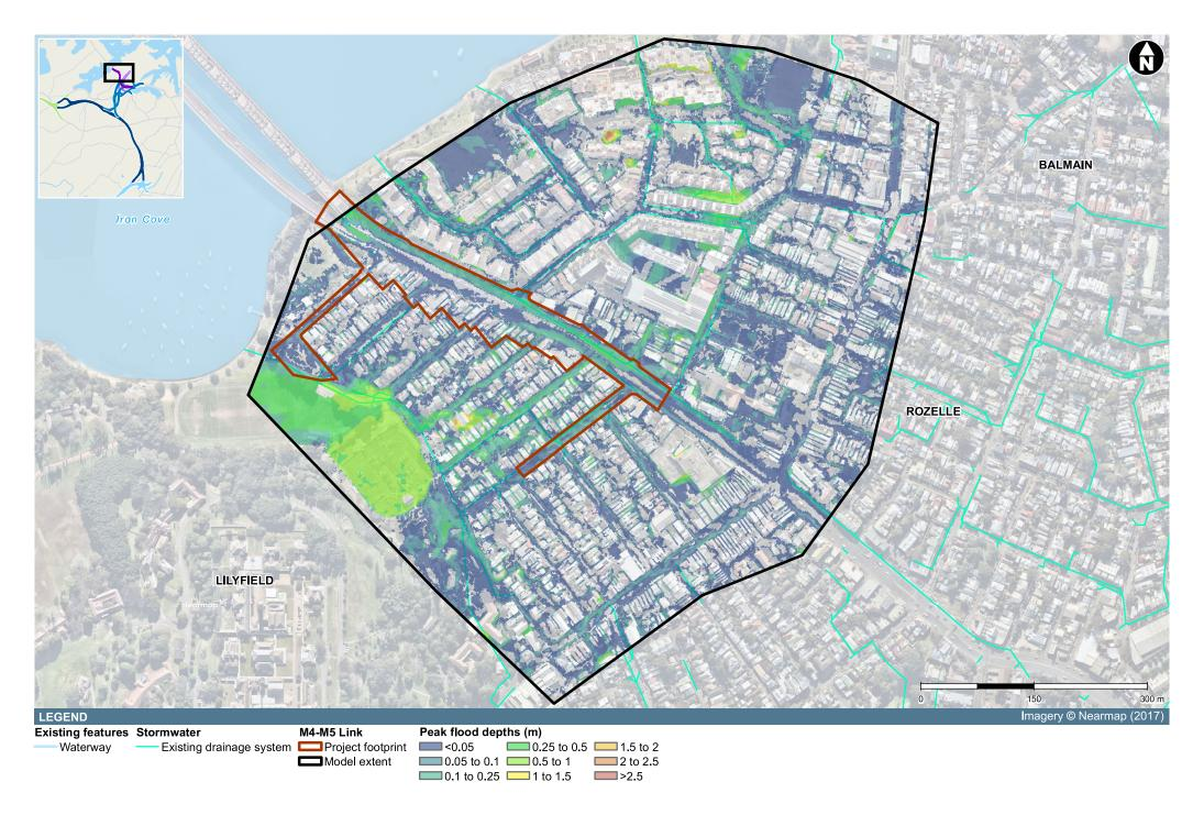
Figure 4-12 Present day flood behaviour – Iron Cove Link - peak flood depths (PMF)
