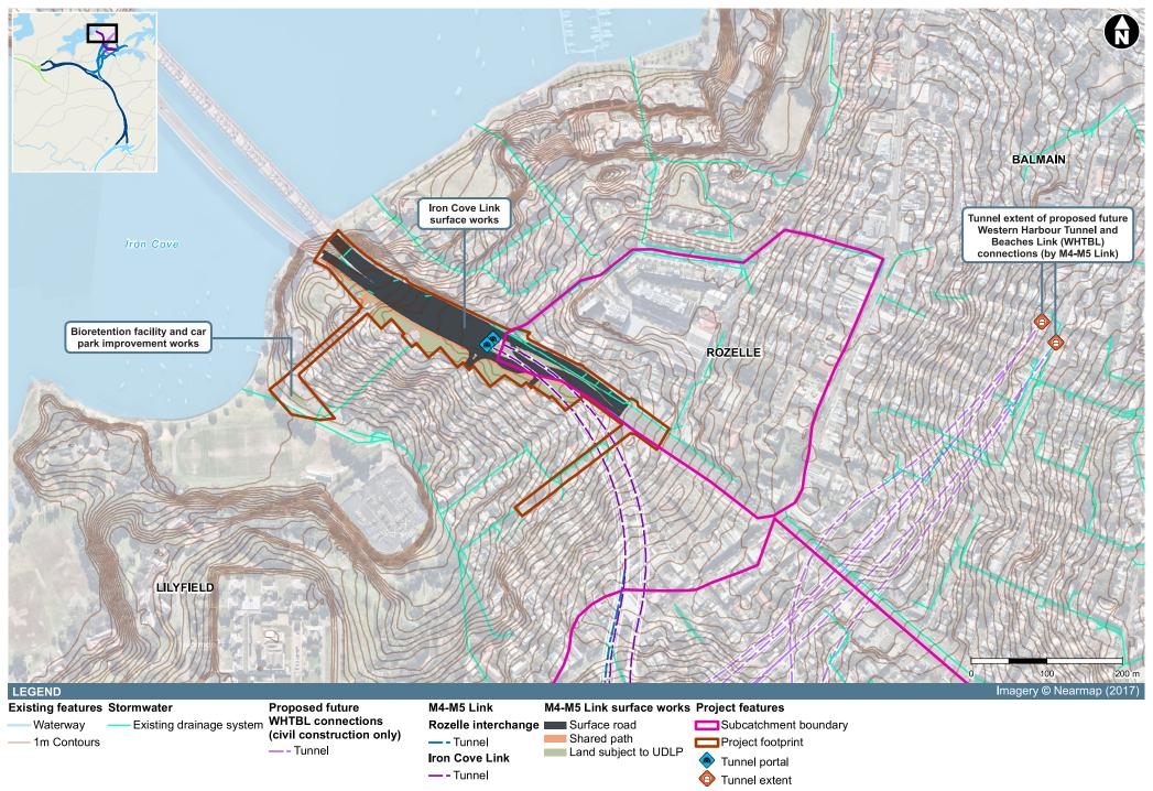
Figure 4-9 Subcatchment draining to Iron Cove Link civil site
