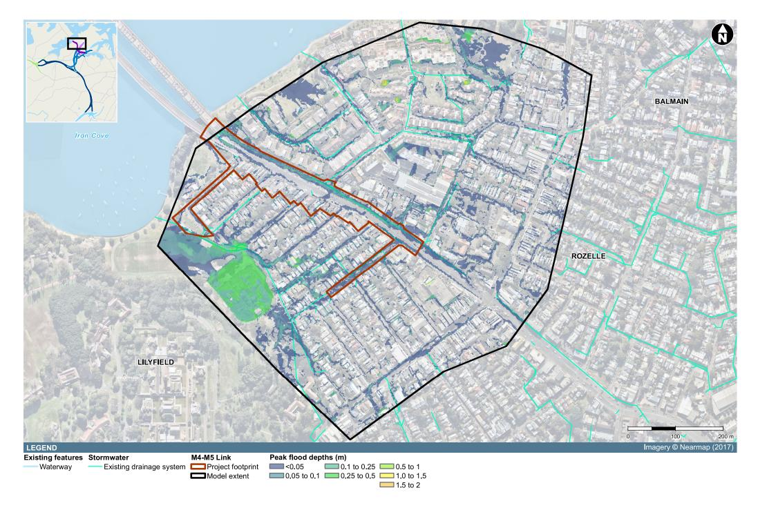
Figure 4-10 Present day flood behaviour – Iron Cove Link - peak flood depths (10 year ARI)
