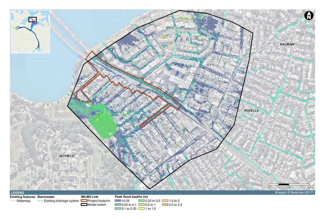
Figure 4-11 Present day flood behaviour – Iron Cove Link - peak flood depths (100 year ARI)
