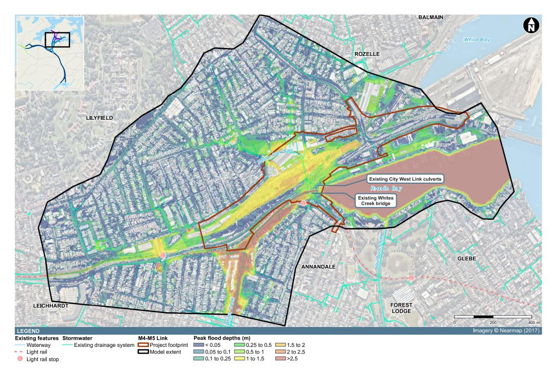
Figure 4-6 Present day flood behaviour – Rozelle interchange - peak flood depths (PMF)
