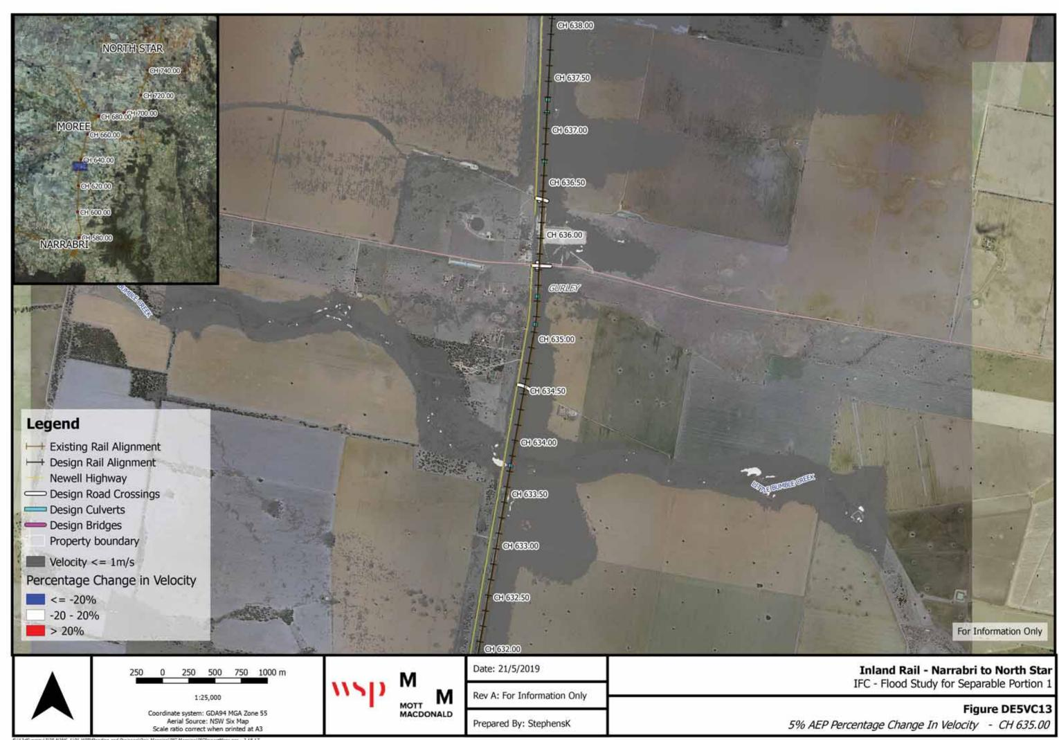
N2NS\_1101 WIP\Flooding and Drainage1Qgis Map
