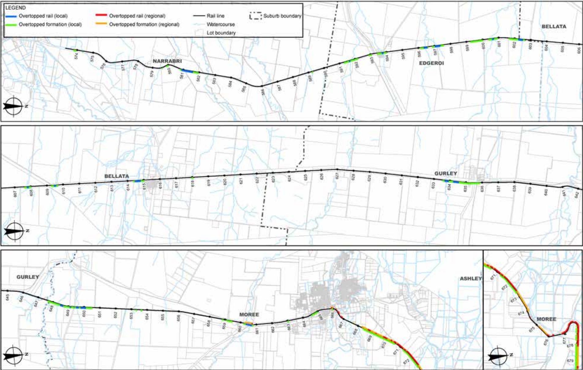
Figure 15.2a Existing rail overtopping locations for 1% AEP event – local and regional catchment flooding
