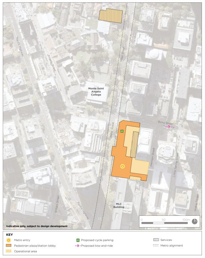
Figure 2-3 Victoria Cross Station - location and indicative layout
