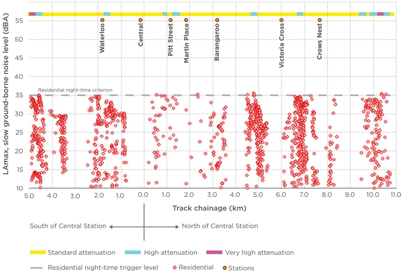
Figure 11-3 Predicted ground-borne noise levels – residential receivers
