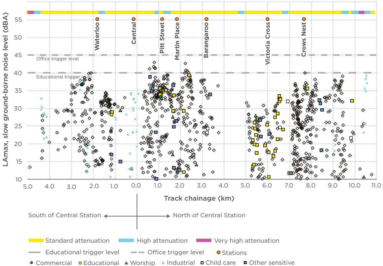
Figure 11-4 Predicted ground-borne noise levels – commercial and other sensitive receivers
