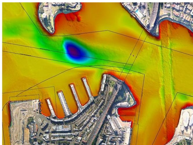
Figure 20 45m deep hole located to the east of the Project area (Sydney Ports n.d).
