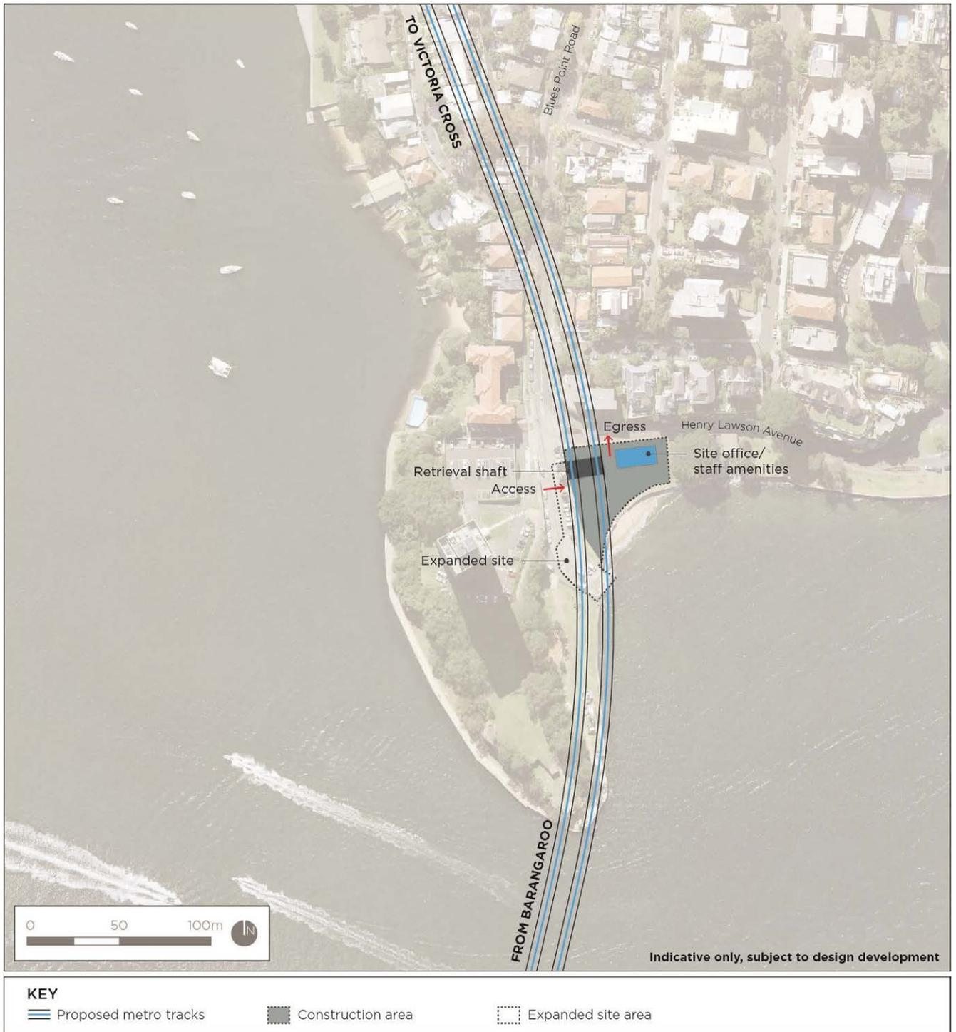
Figure 3.13 : Layout of the Blues Point temporary site
