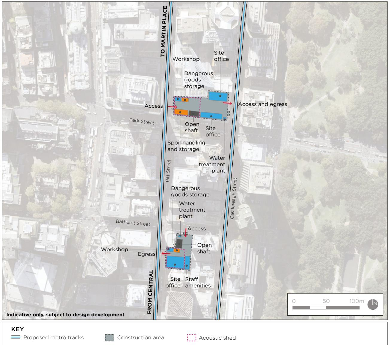
Figure 7-15 Pitt Street Station construction sites indicative layout
