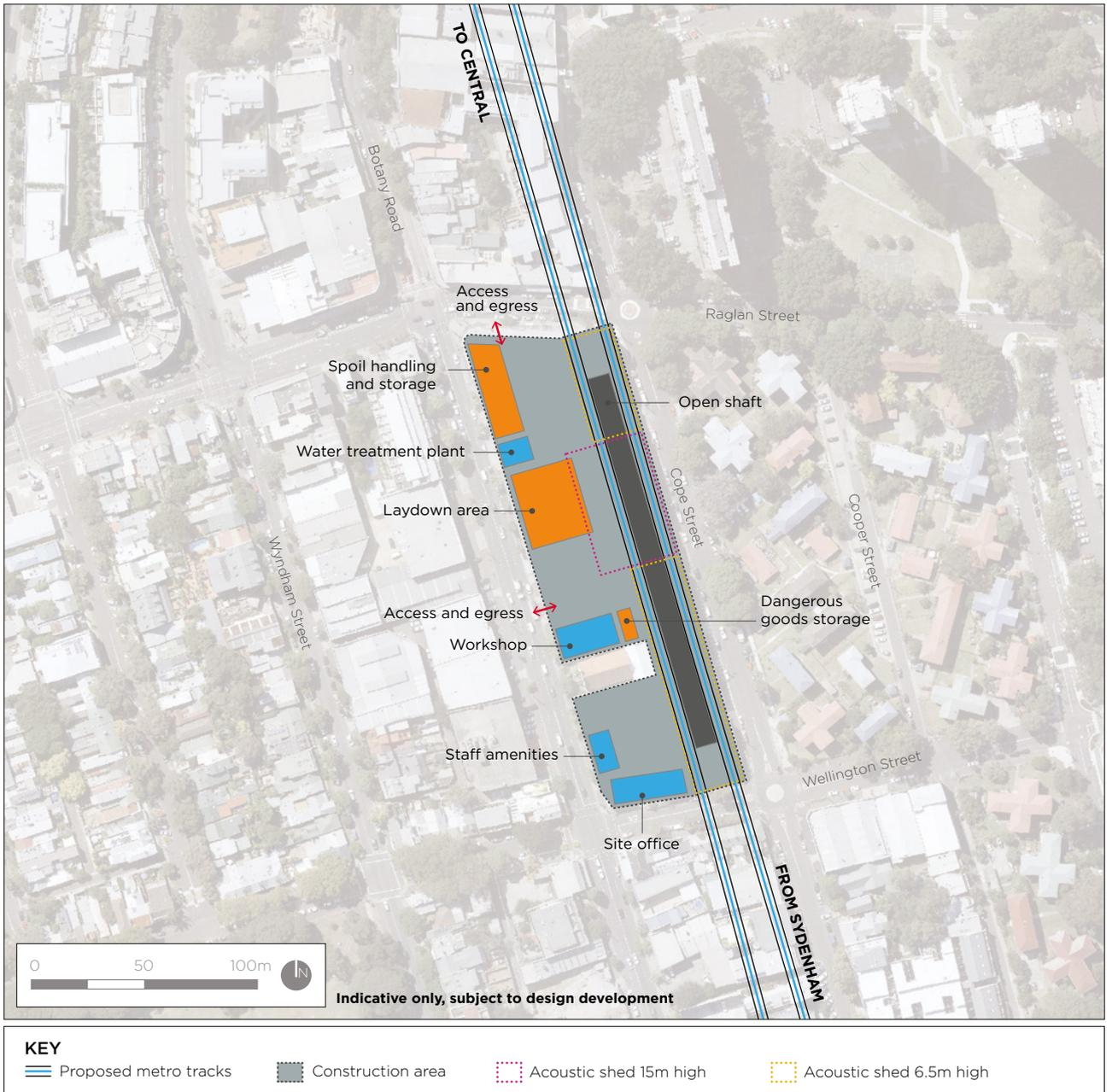
Figure 7-20 Waterloo Station construction site indicative layout
