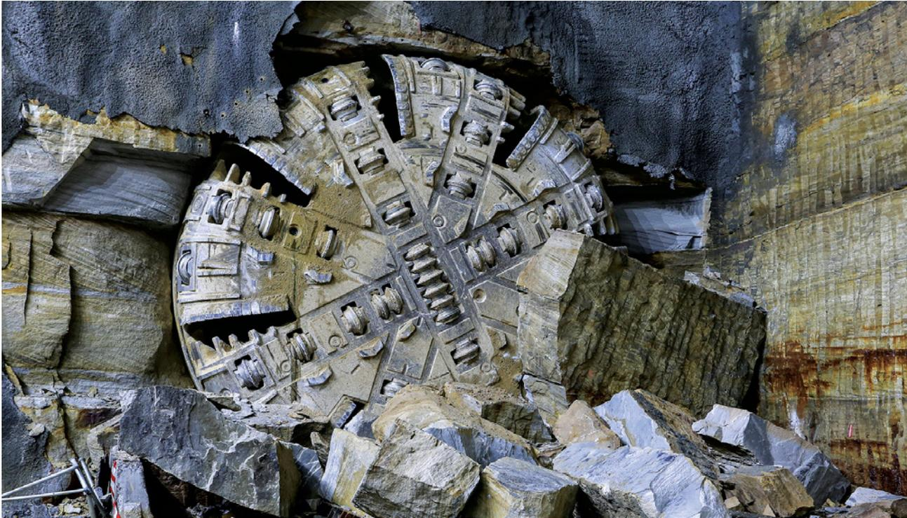
Photo of a tunnel boring machine cutter head
