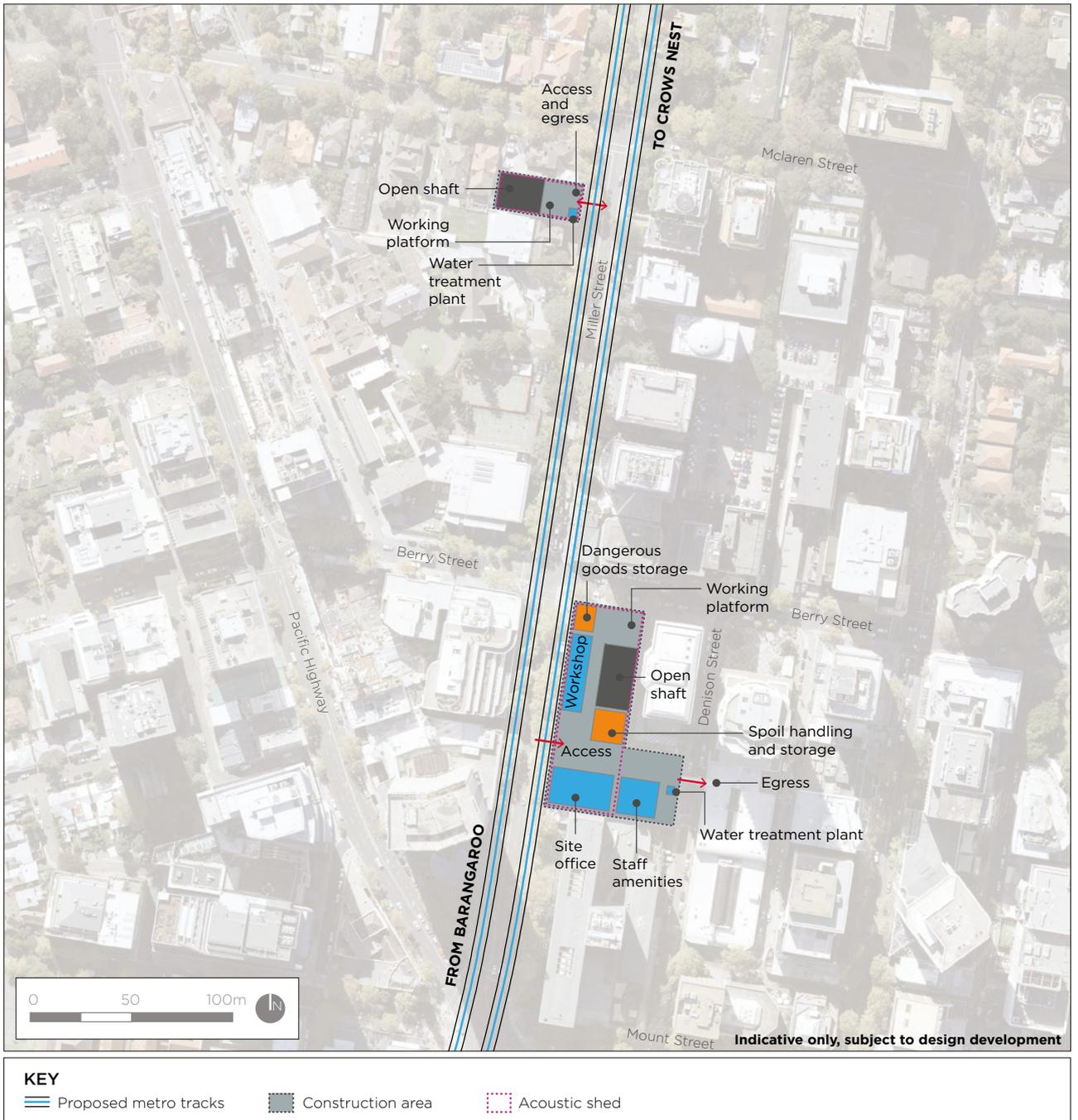
Figure 7-11 Victoria Cross Station construction site indicative layout
