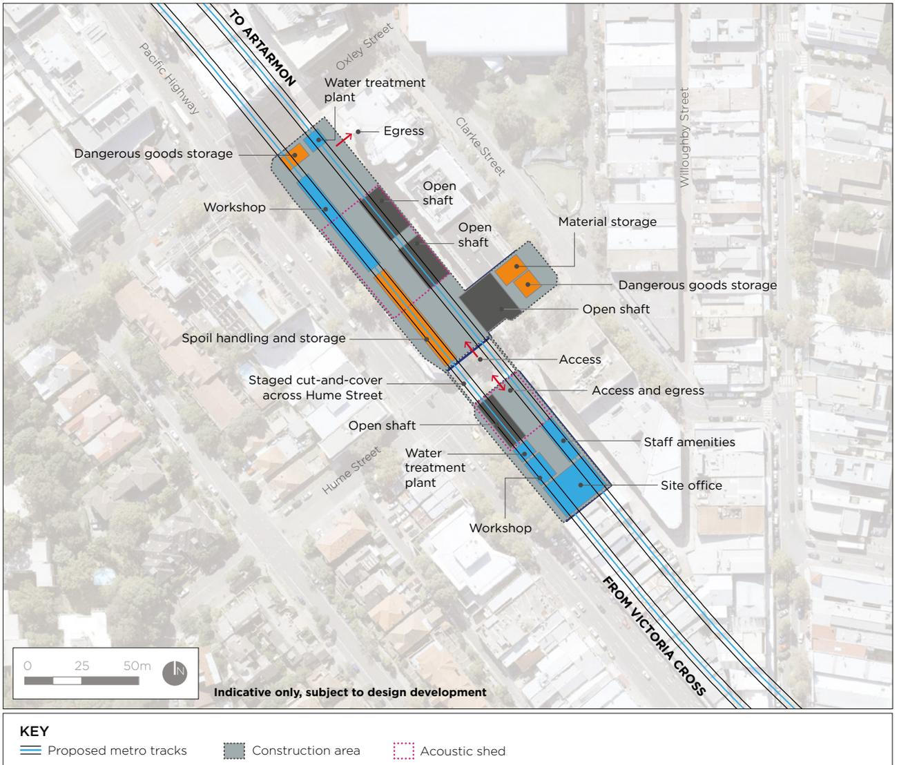
Figure 7-10 Crows Nest Station construction site indicative layout
