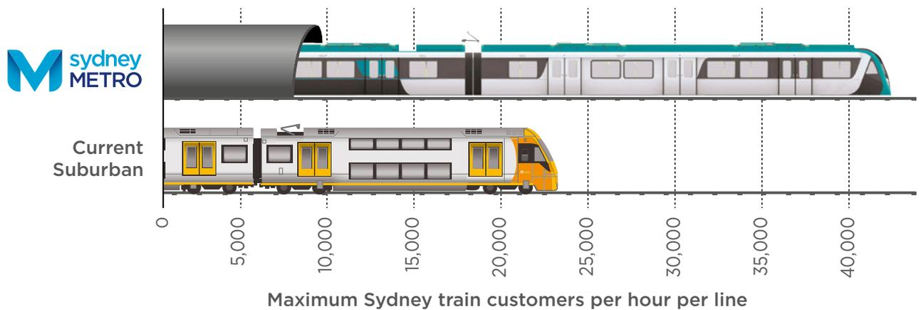
**Figure 3-9** Line capacity comparison between Sydney Trains and Sydney Metro networks
