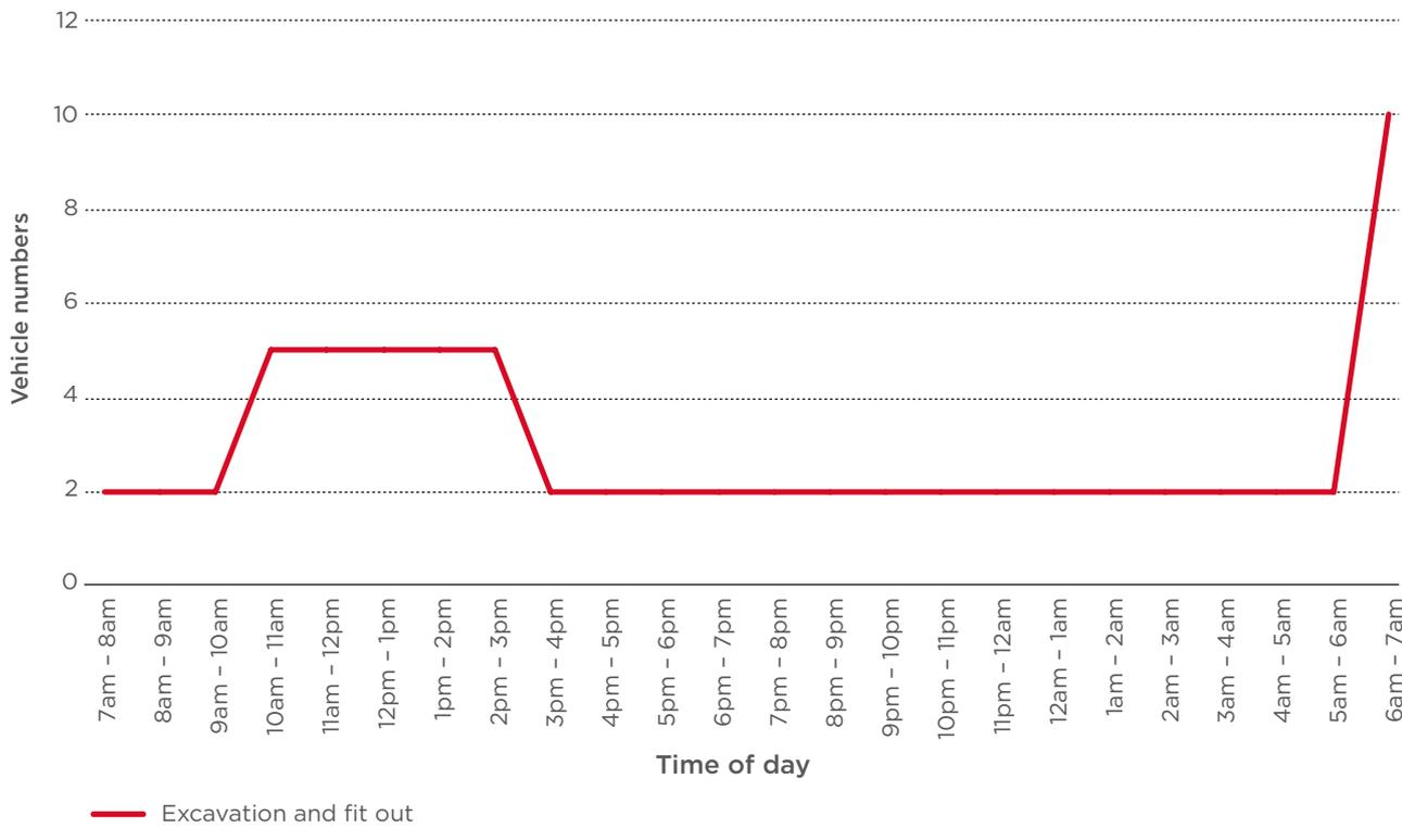
Figure 3-13 O’Connell Street construction site – hourly traffic profile of construction vehicles (inbound only)
