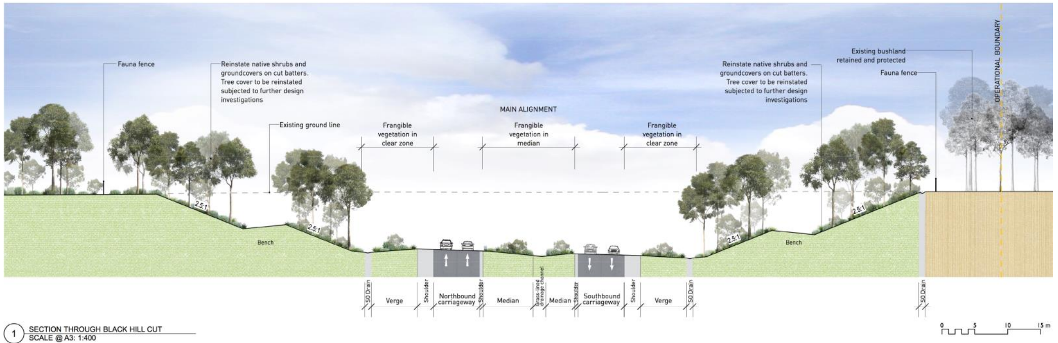
Figure 15-4 Cross section (indicative only) at Black Hill cut, about 700m east of the existing M1 Pacific Motorway at Black Hill
