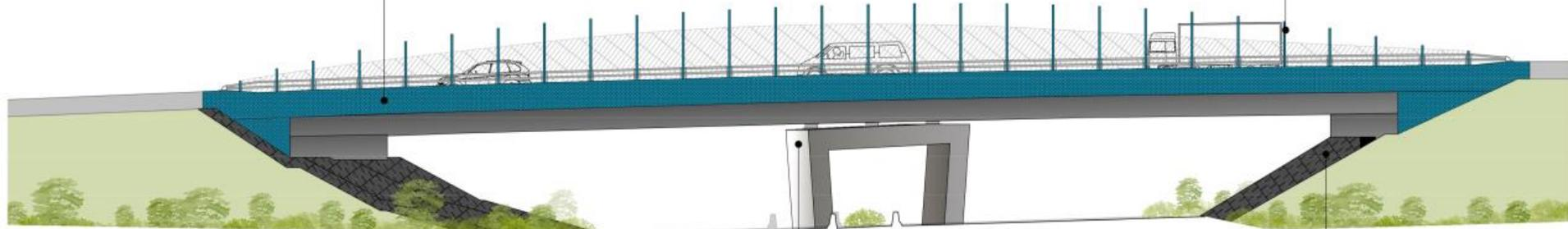
Typical elevation of Type 1 bridge over M1 Pacific Motorway showing proposed urban design outcomes. For specific bridge elevations refer Section 6.12.3
