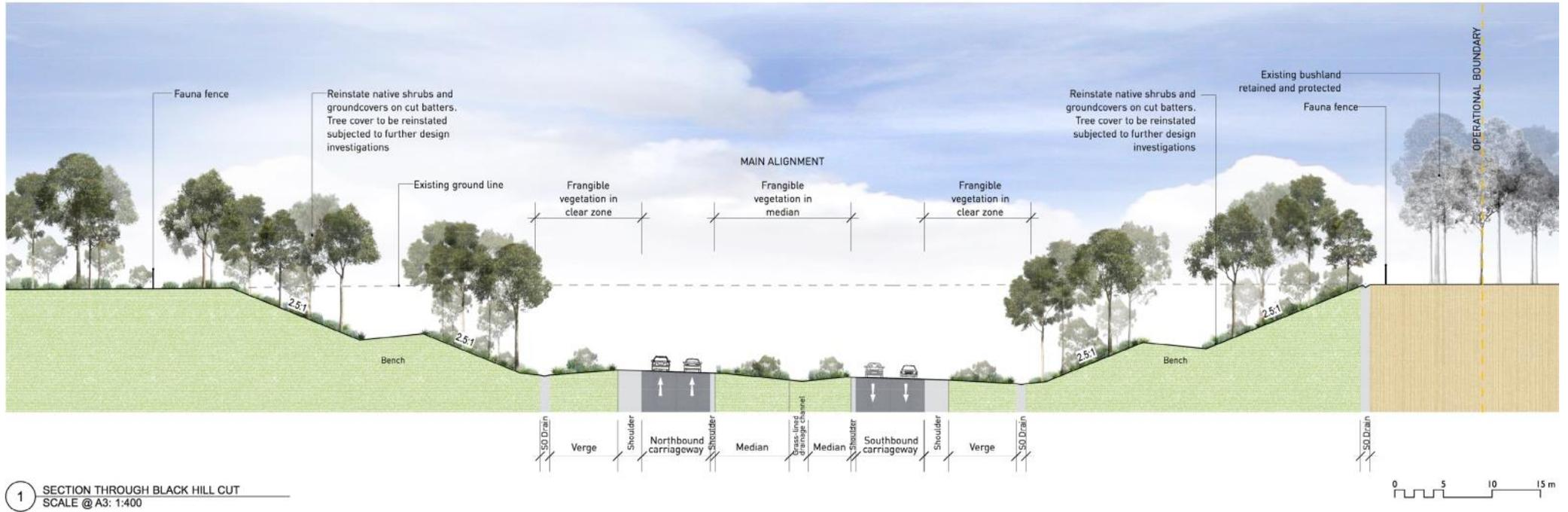
Figure 15-4 Cross section (indicative only) at Black Hill cut, about 700m east of the existing M1 Pacific Motorway at Black Hill
