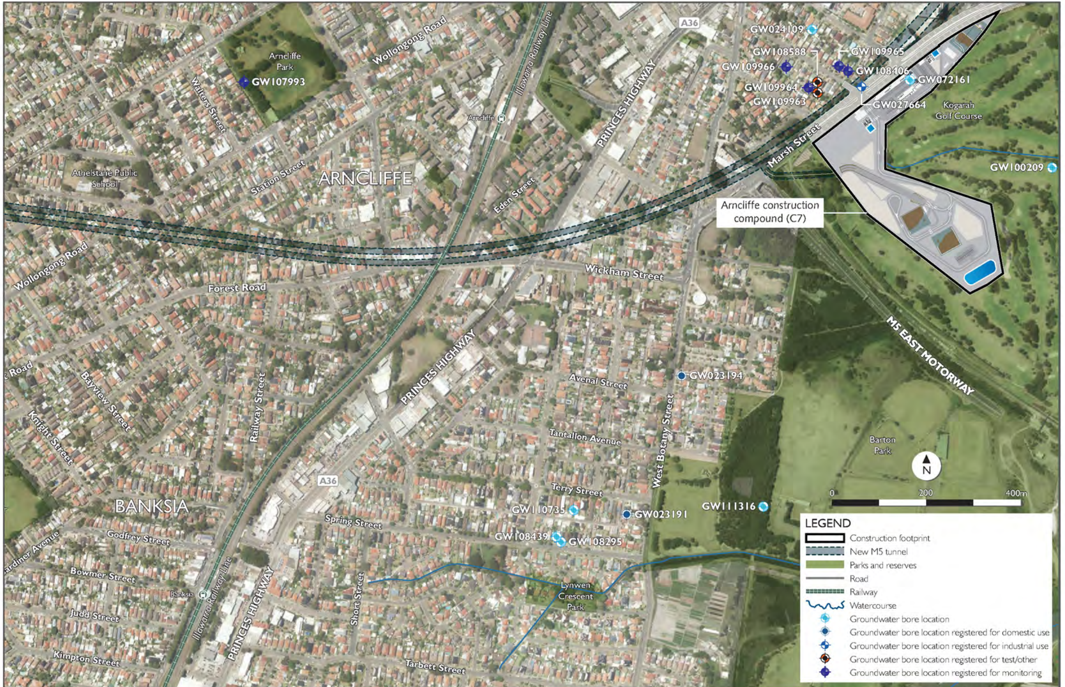
Figure 7-4 Registered boreholes predicted to be impacted - Arncliffe surface works
