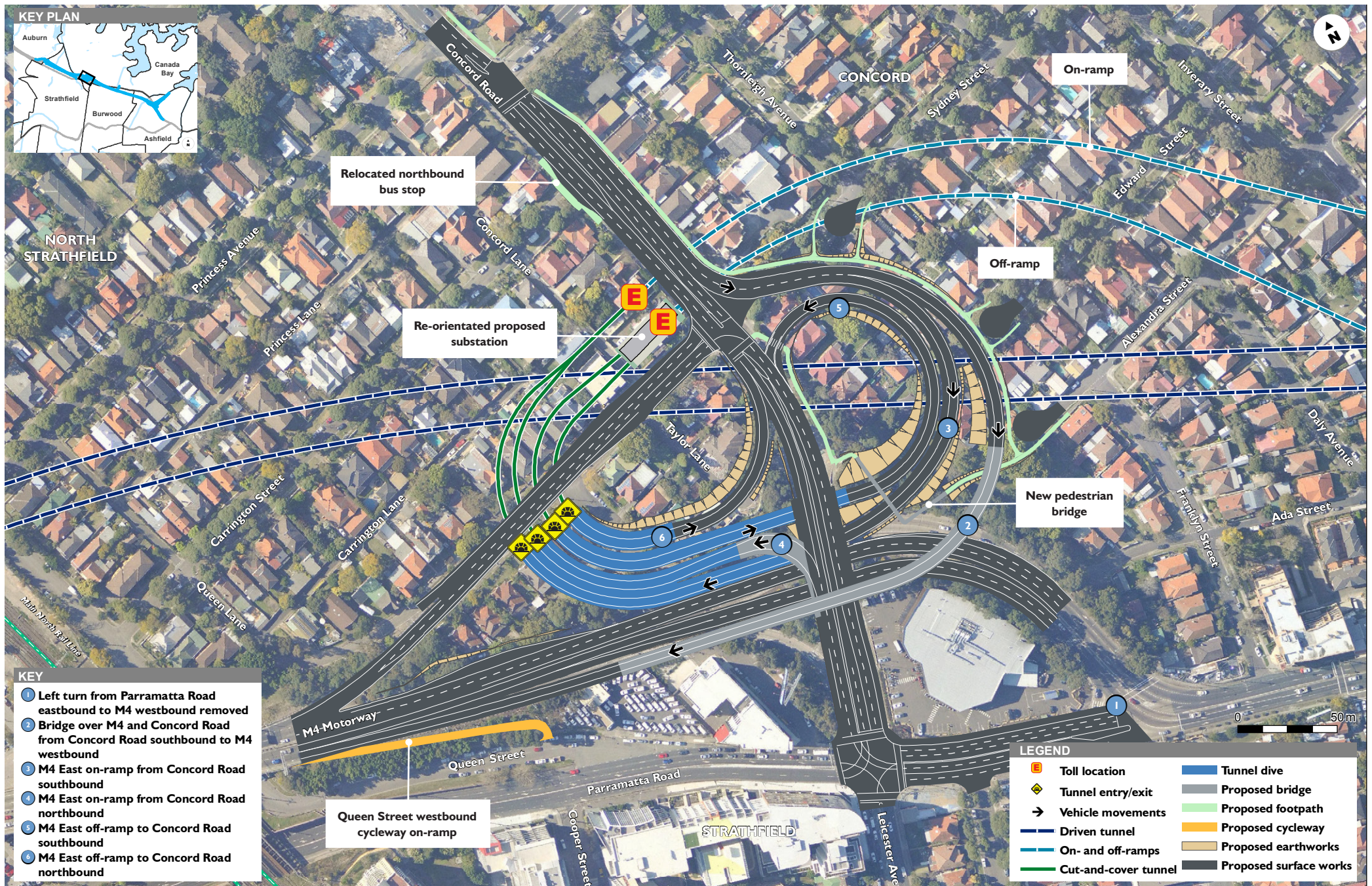
Figure 2.9 Change in orientation of Sydney Street substation
