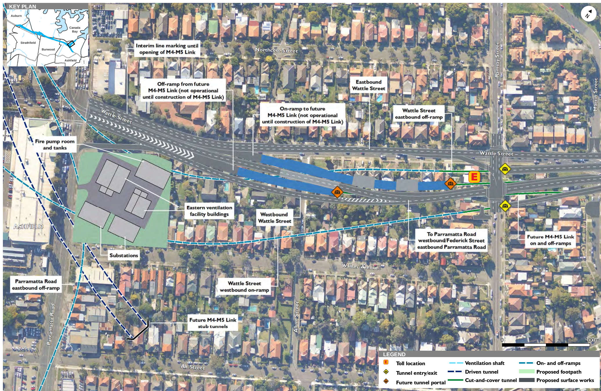
Figure 2.1 Reconfigured Wattle Street (City West Link) interchange
