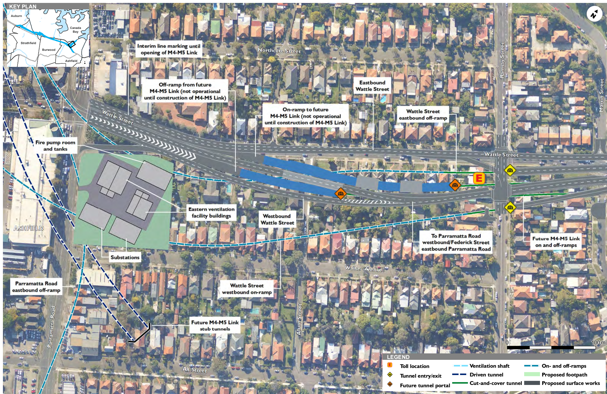
Figure 2.1 Reconfigured Wattle Street (City West Link) interchange
