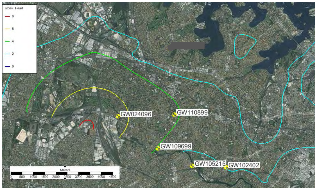
Figure 6.32 Run 107 layer 4 steady-state piezometric contours, standard deviation (metres) of all stochastic runs.
