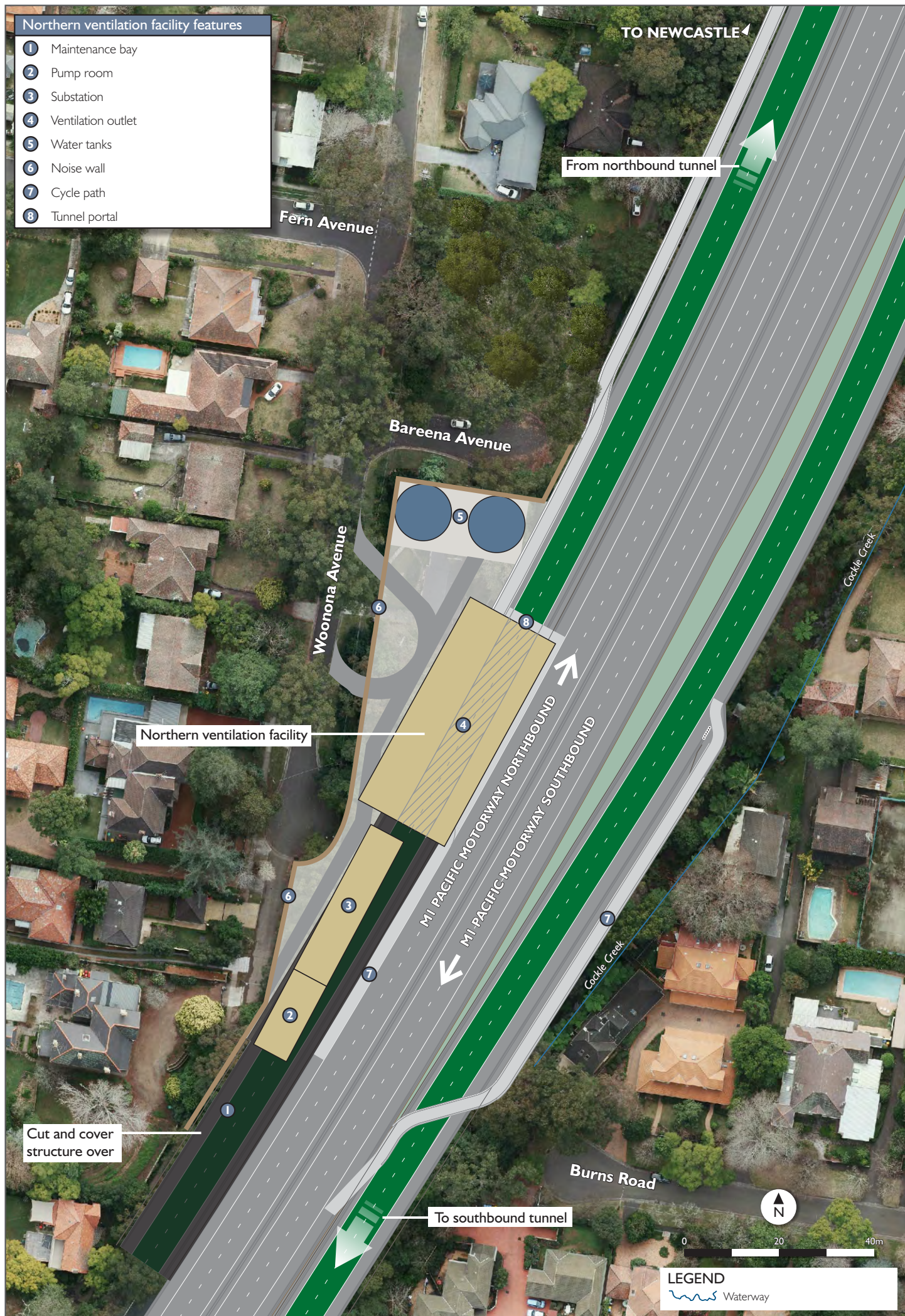
Figure 5-18 Northern ventilation facility operational layout
