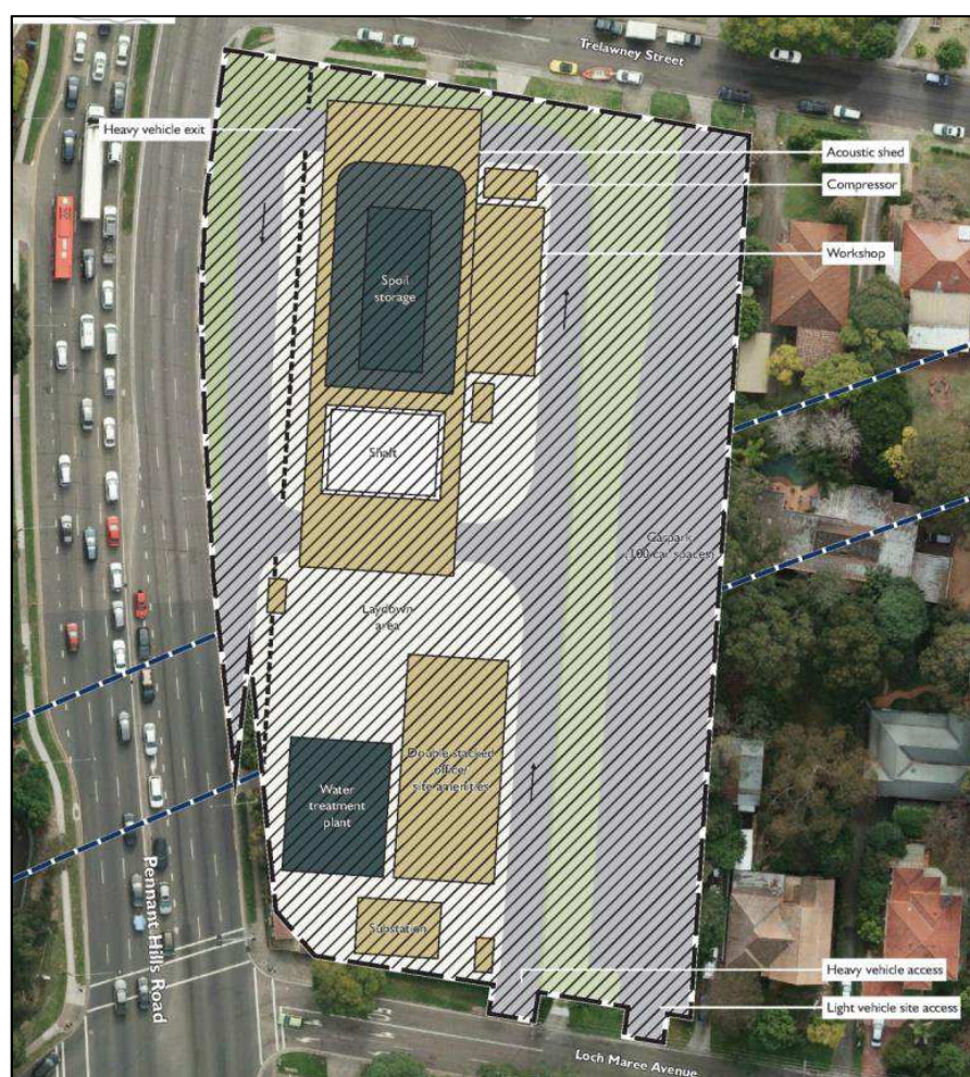
Figure 17: Trelawney Street construction compound Source: Environmental Impact Statement
