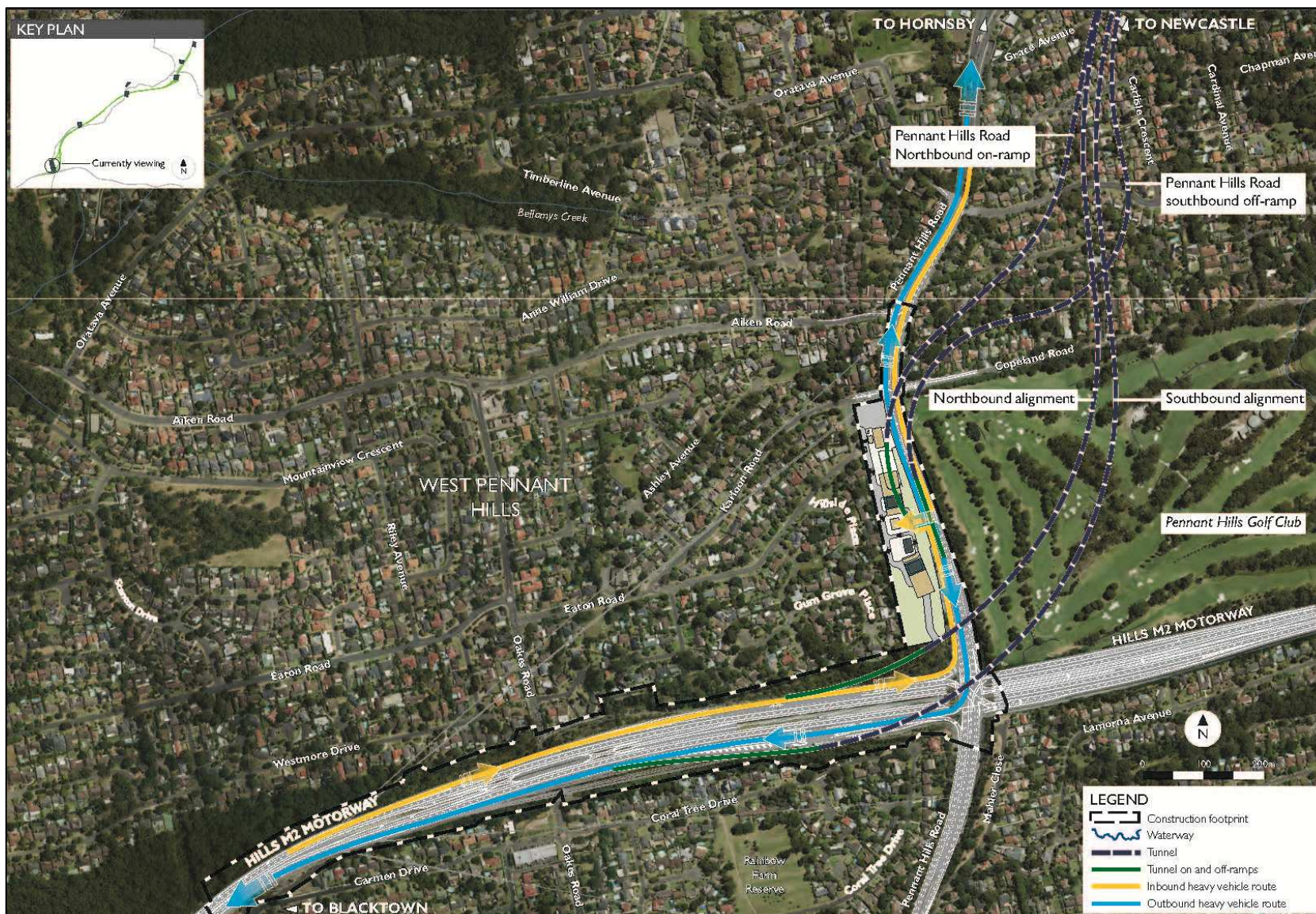
Figure 11: Southern interchange compound access arrangement C5-1. Source: Response to Submissions Report
