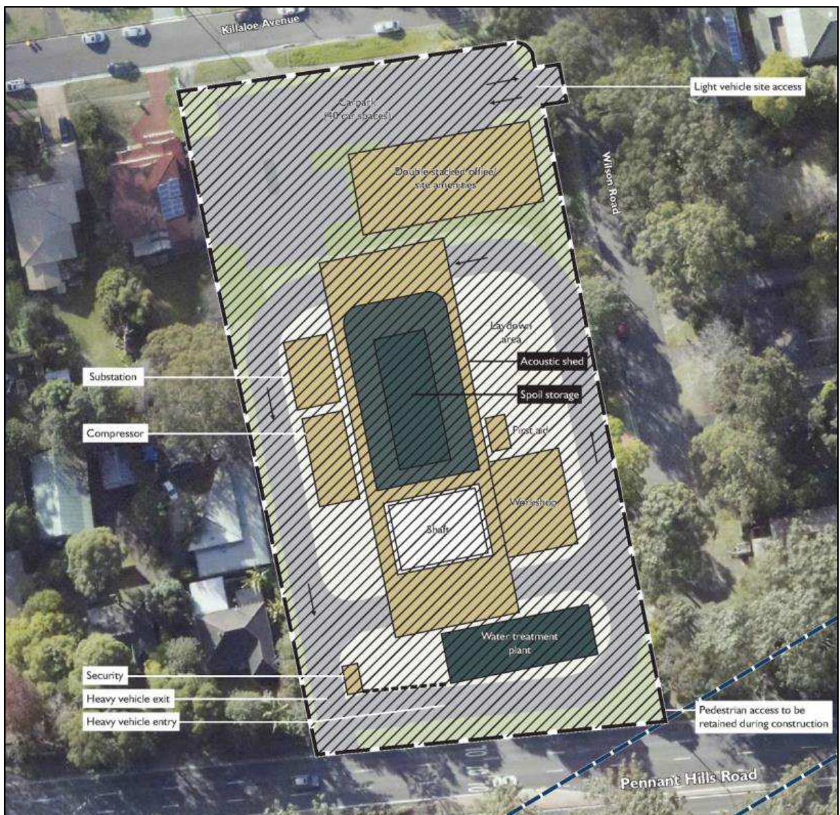
Figure 16: Wilson Road construction compound Source: Environmental Impact Statement .
