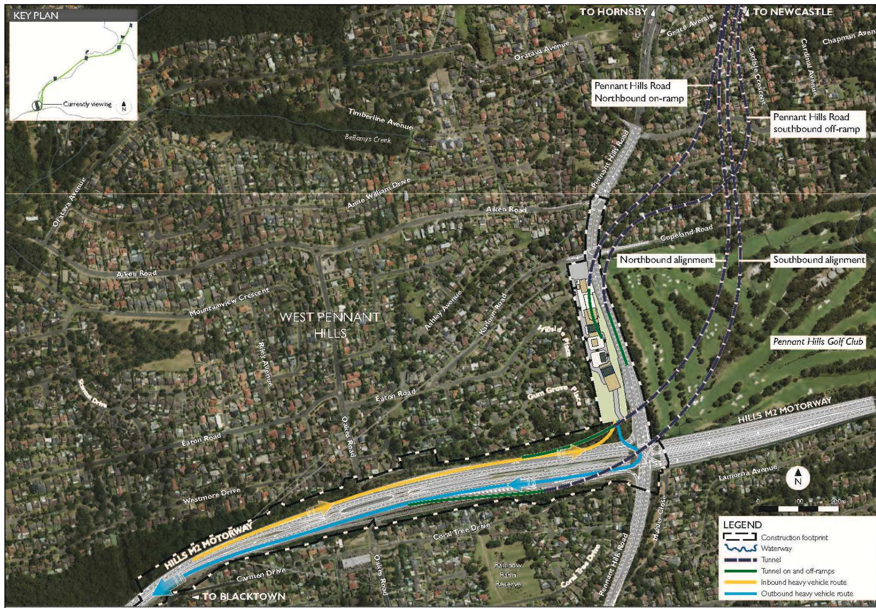
Figure 15: Southern interchange compound access arrangement C5-2. Source: Response to Submissions Report
