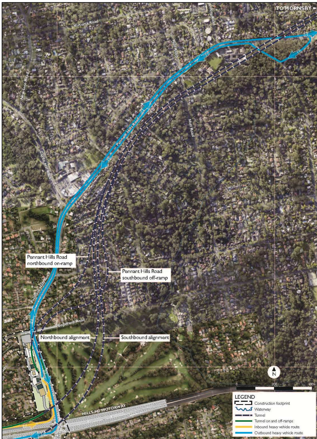
Figure 12: Southern interchange compound access arrangement C5-3. Source: Response to Submissions Report
