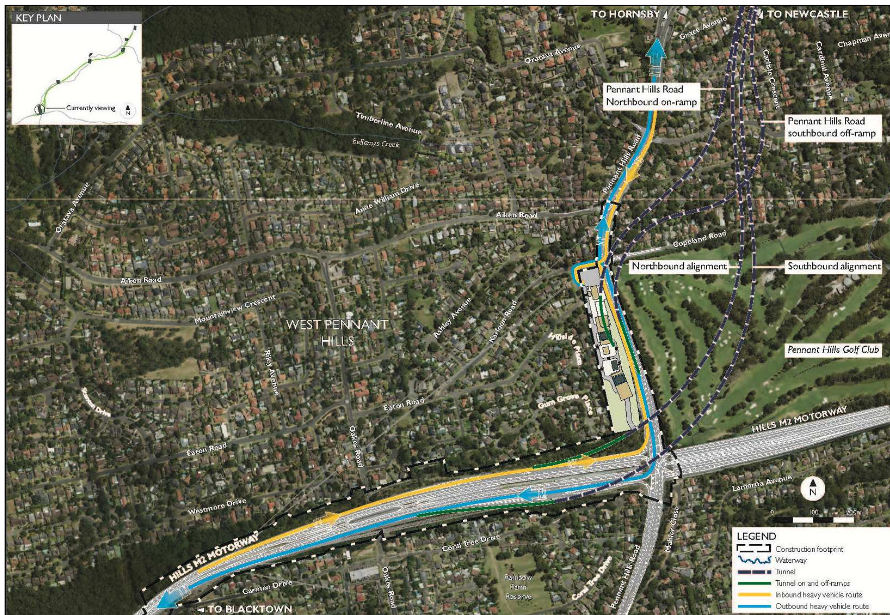
Figure 14: Southern interchange compound access arrangement C5-5. Source: Response to Submissions Report
