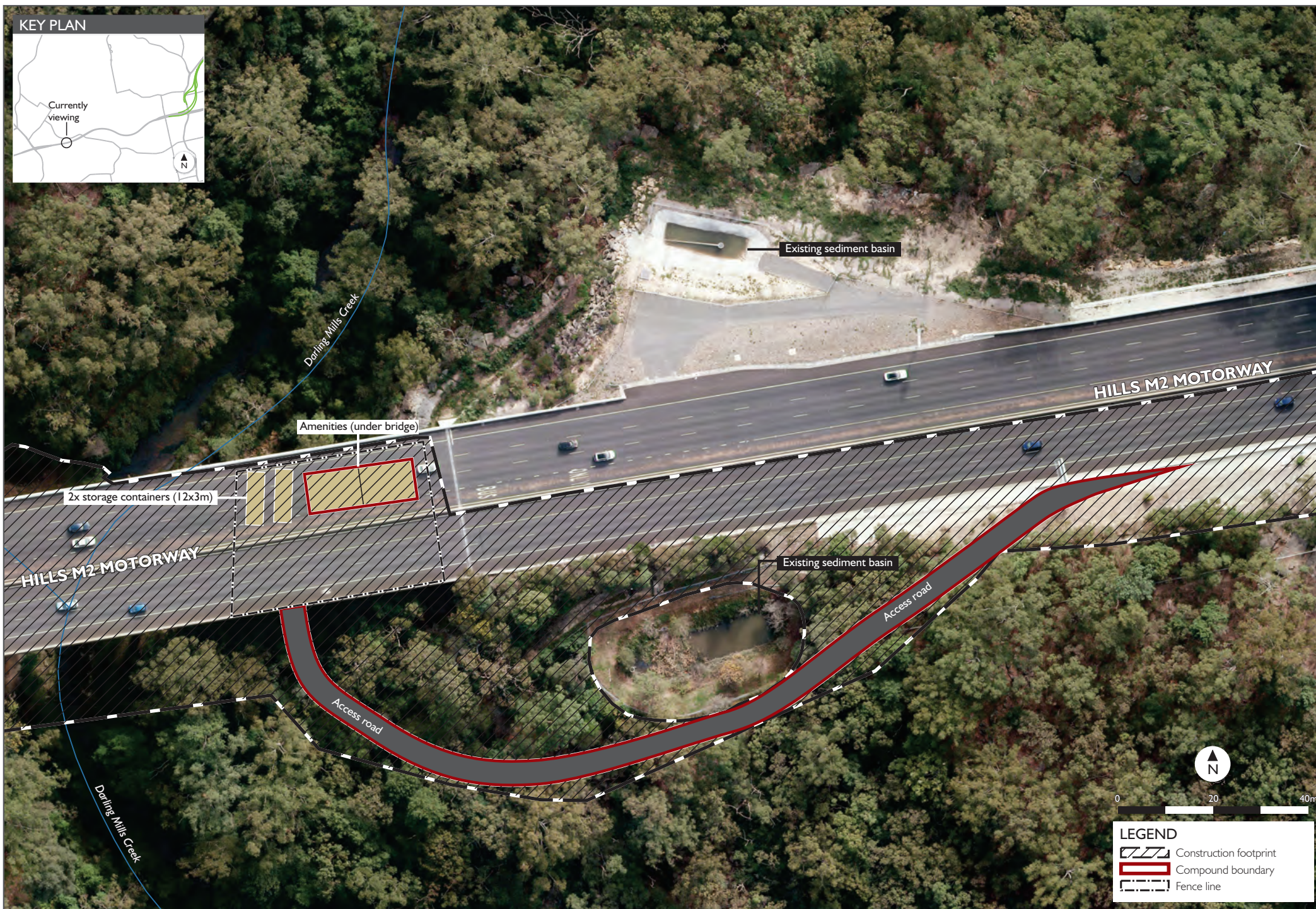
Figure 4-2 Indicative Darling Mills Creek viaduct construction compound revised layout
