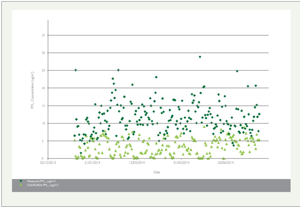
Figure 2-18 CAL3QHCR validation - Observatory Park PM<sub>2.5</sub> (24 hour)
