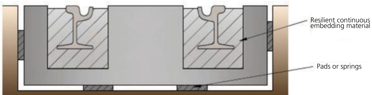
Very high attenuation floating slab with embedded rail
