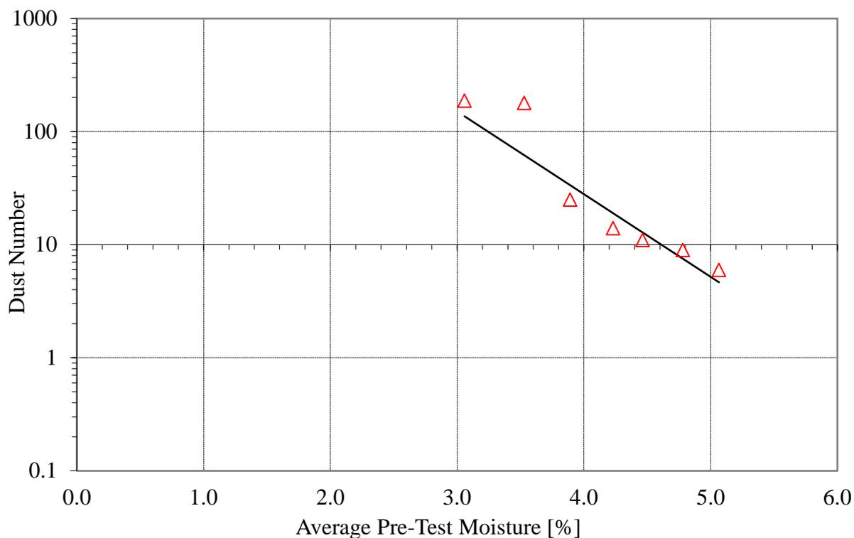
**Figure 2** Dust number measurement results for Wongawilli ROM Coal -6.3mm.
