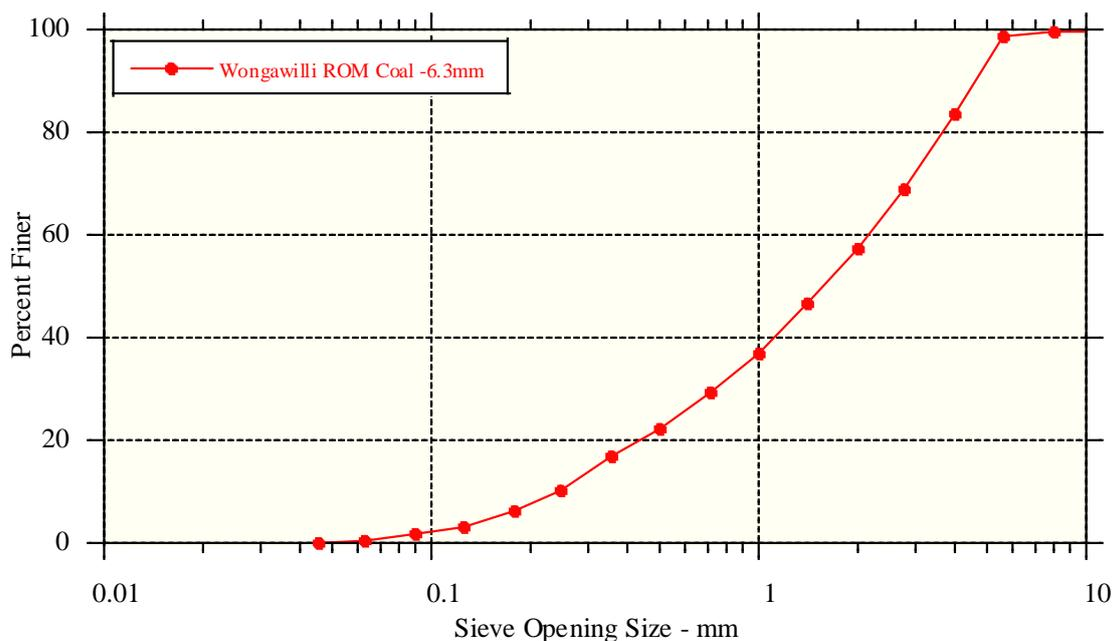
**Figure 1** Particle size distribution for Wongawilli ROM Coal -6.3mm.
