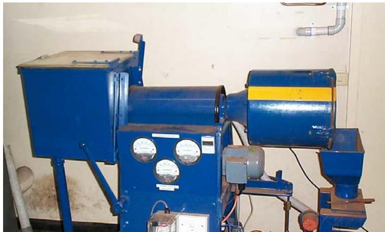
Figure 1 – Dust Extinction Moisture Test Facility
