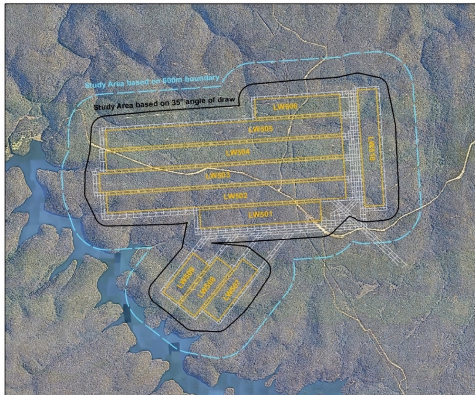
Fig. 0.2 Aerial photograph showing the proposed longwalls and the Study Area
