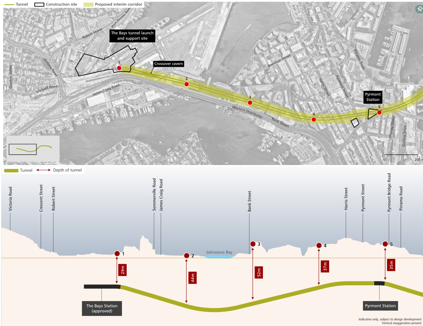
Figure 5 Indicative alignment plan and long section of tunnel (Page 1)
