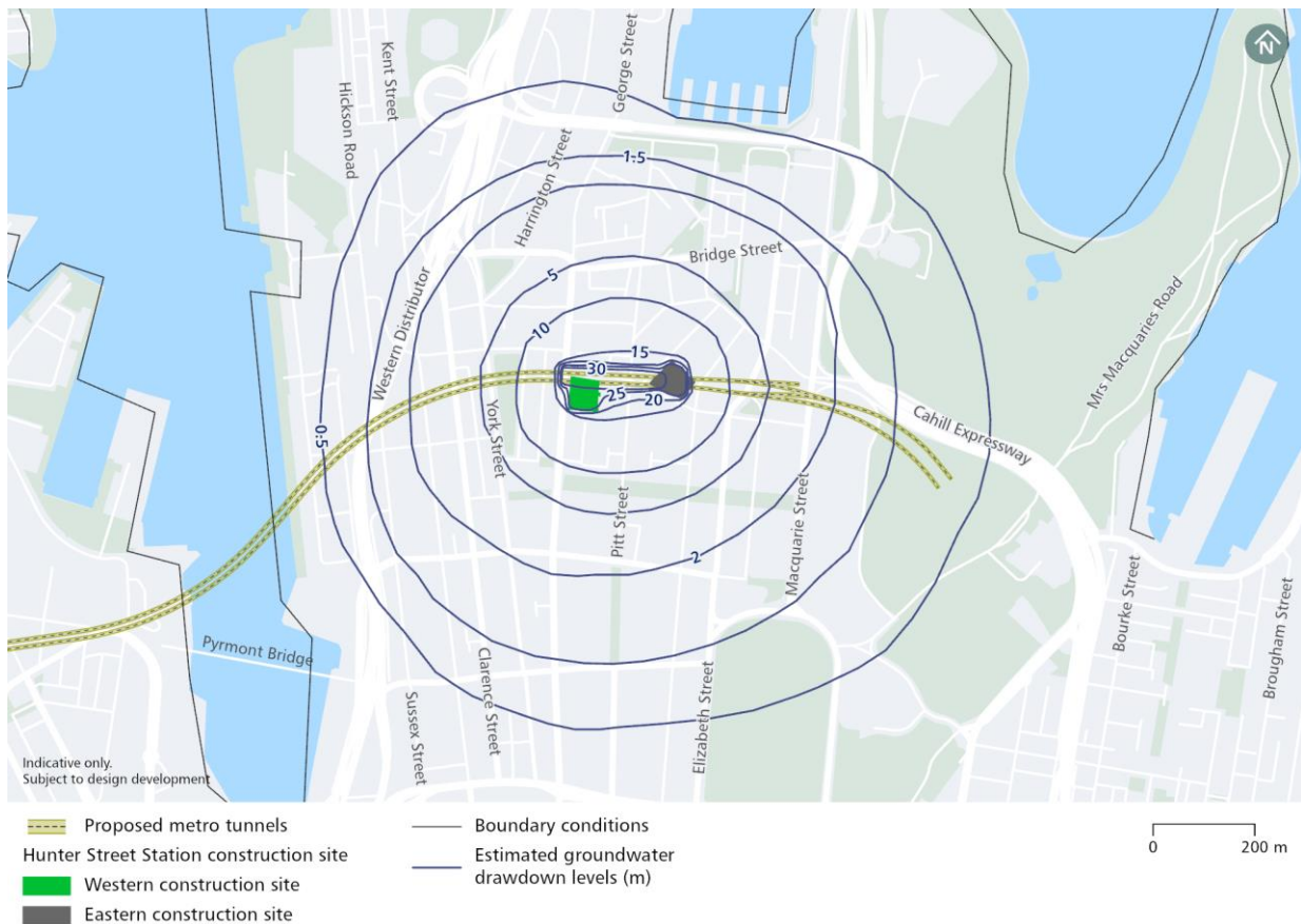
Figure 5-6: Estimated drawdown after 2 years due to excavation – Hunter Street Station (Sydney CBD)
