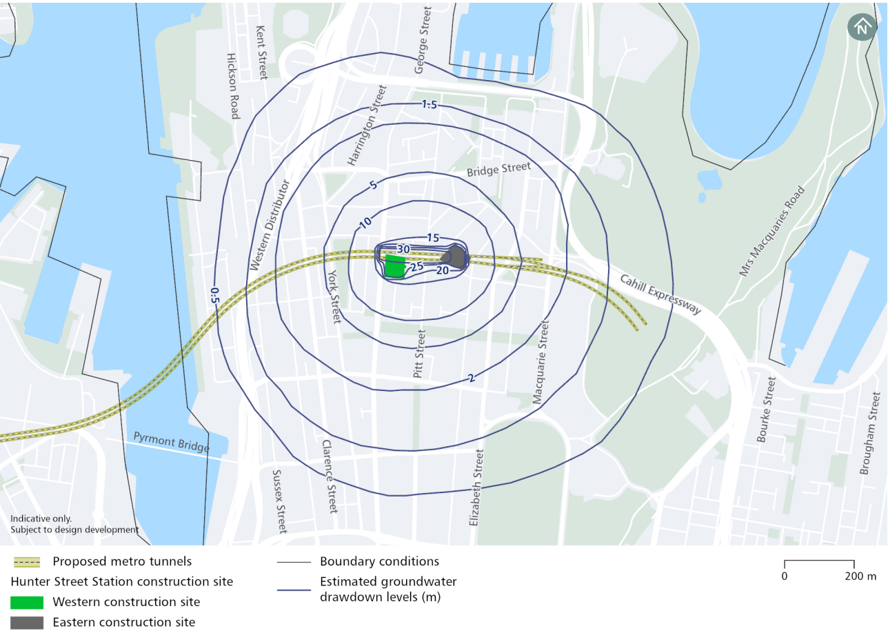
Figure 14-5 Estimated groundwater drawdown two years after the start of construction – Hunter Street Station (Sydney CBD) construction sites
