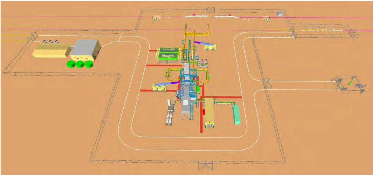
Figure 2.1 Indicative compressor station layout
