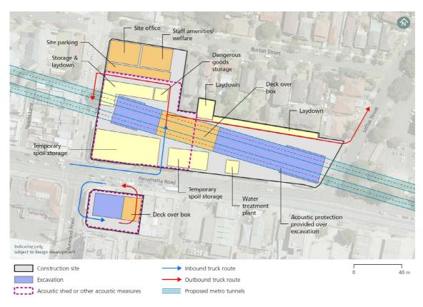
Figure 2-7: Burwood North Station construction site
