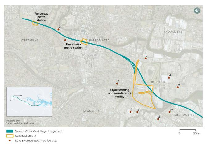
Figure 3-7: NSW EPA regulated / formerly regulated / notified sites within 500 metres of the construction footprint and alignment – Map 1
