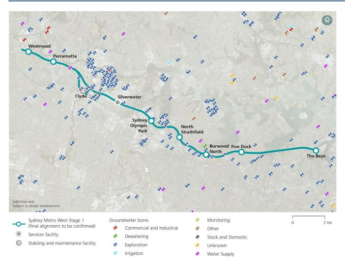
Figure 3-6: WaterNSW-registered groundwater bores along the Stage 1 alignment
