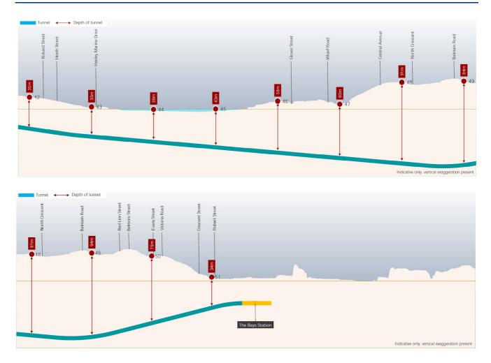
Figure 3-3: Tunnel alignment and depths – Five Dock to The Bays
