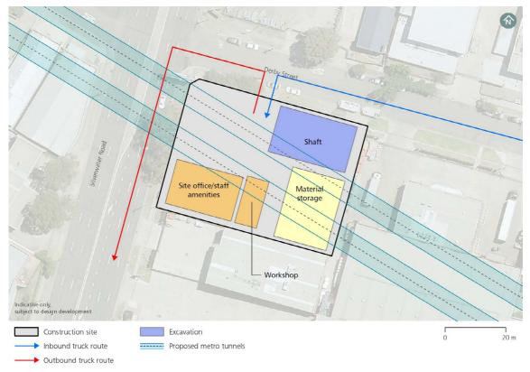
Figure 2-4: Silverwater services facility construction site
