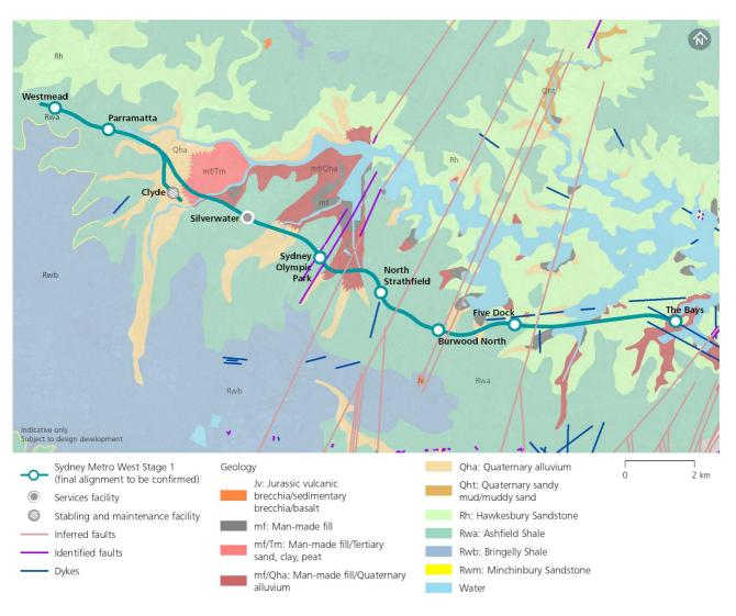
Figure 3-4: Geology along the Stage 1 alignment
