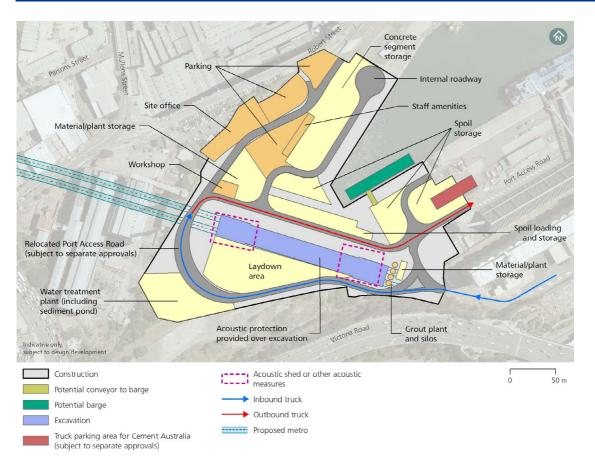
Figure 2-9: The Bays Station construction site
