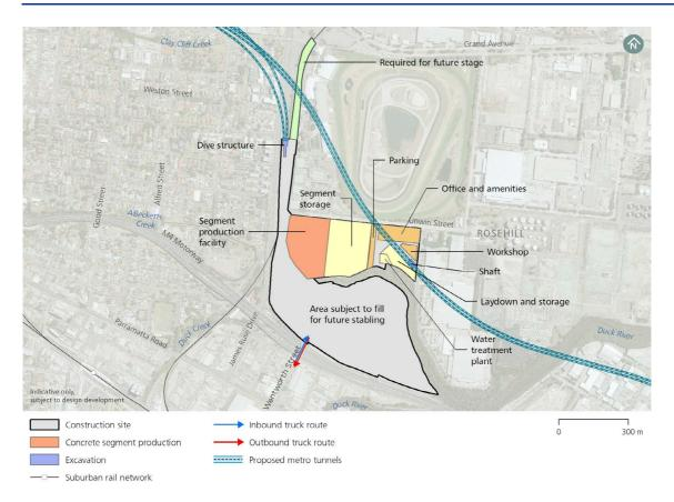
Figure 2-3: Clyde stabling and maintenance facility construction site
