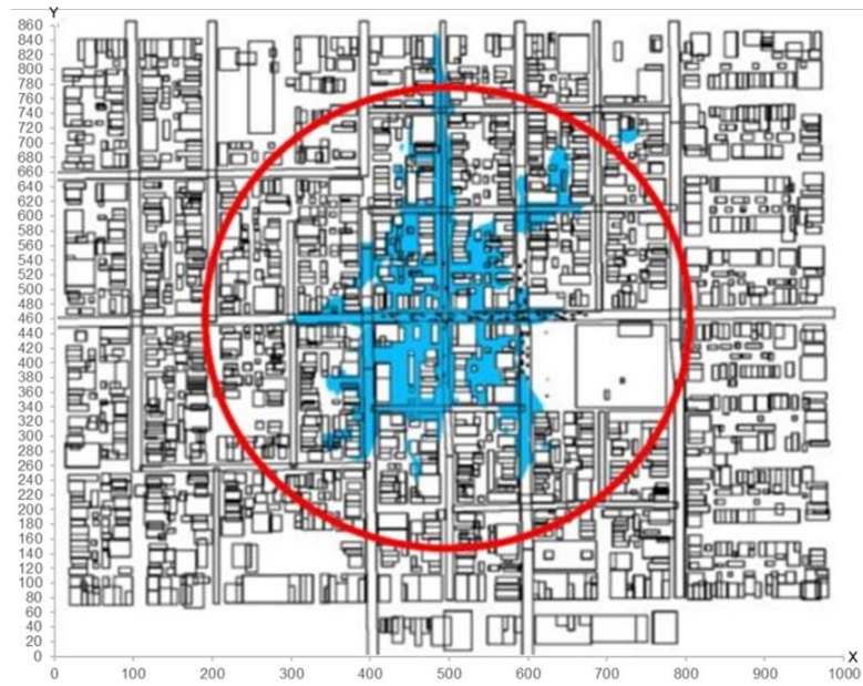
Figure 11 - Dense gas dispersion for simple dispersion model (red) vs CFD (blue), 2m/s wind (8 directions)
