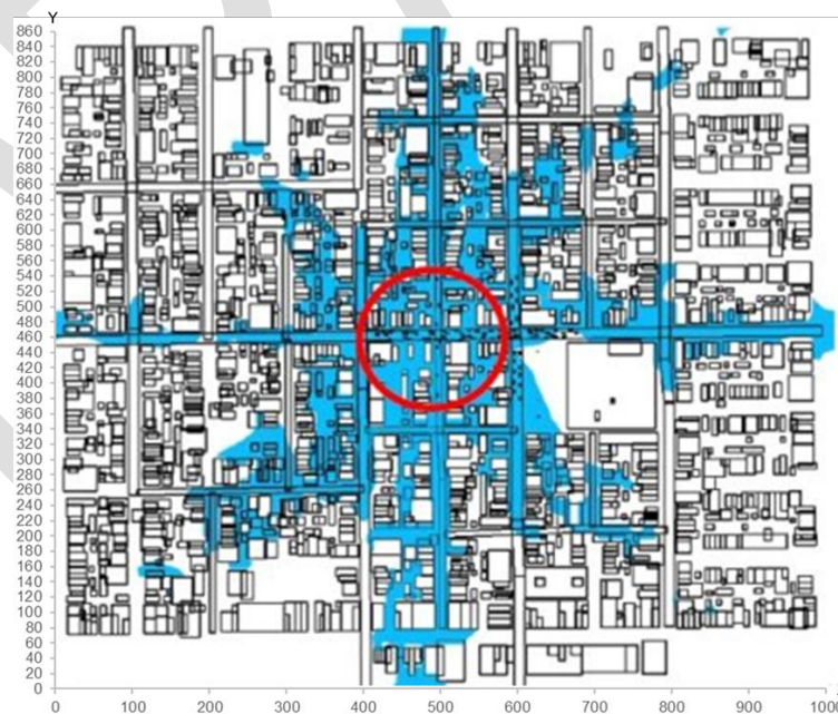
Figure 12 Dense gas dispersion for simple dispersion model (red) vs CFD (blue), 8m/s wind (8 directions)
