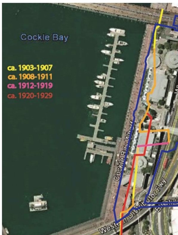
Figure 40: Overlay showing lines of “rat-proof retaining walls” established by the Sydney Harbour Trust in the 1900s-1920s. Study area shown with blue outline.
