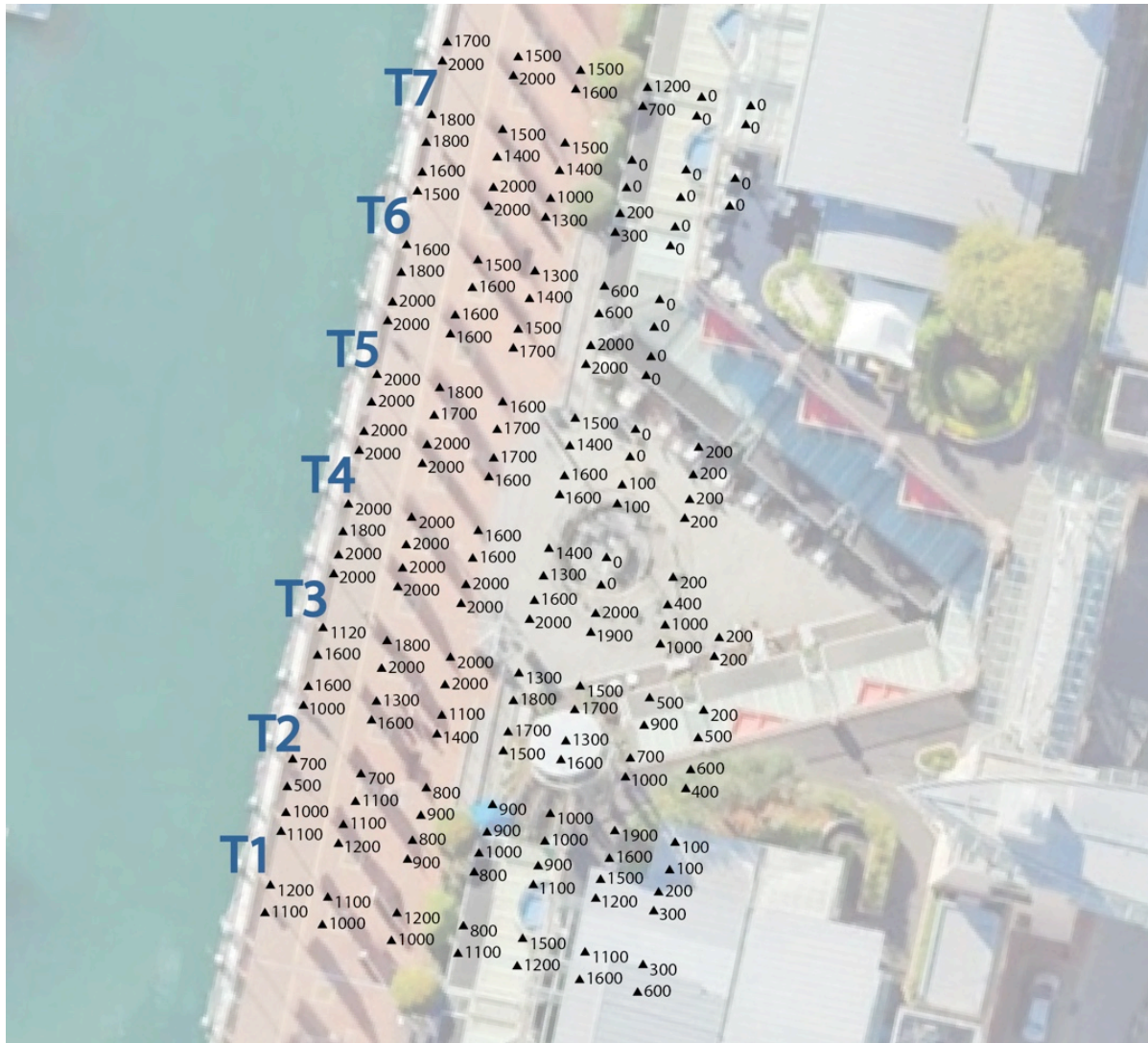
Figure 91: Overlay of probe results along transects in primary survey area. All depths are in mm.
