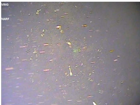
Figure 60: Rubbish and sediment build-up behind rubbish net. (Image from T2 (a) Cockle Bay 210705, 05:53).
