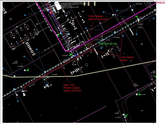
Figure: Existing 132kV and 11kV Underground cables and Proposed Loop in and Out arrangement The figure below shows the 132kV transmission cables and the proposed path for the 11kV cable extension.
