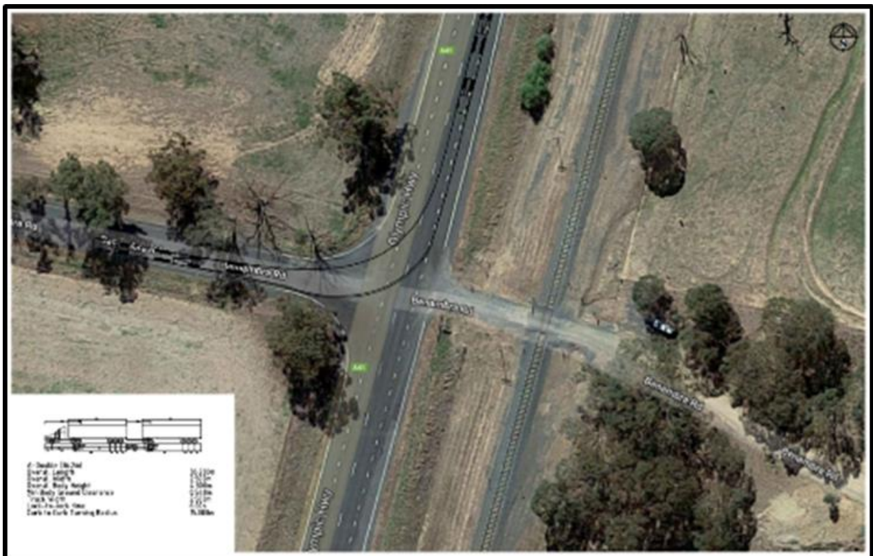
Figure 18 Swept path analysis turning right into Benambra Road
