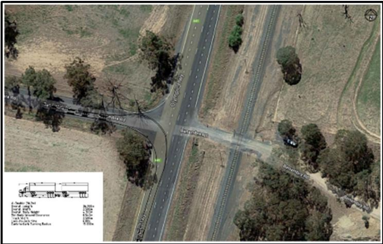
Figure 19 Swept path analysis turning left into Benambra Road
