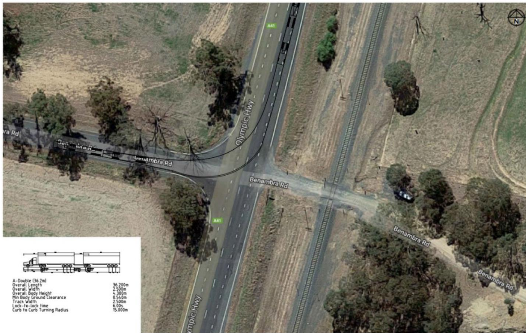
Figure 3-14 Swept path analysis turning right into Benambra Road
