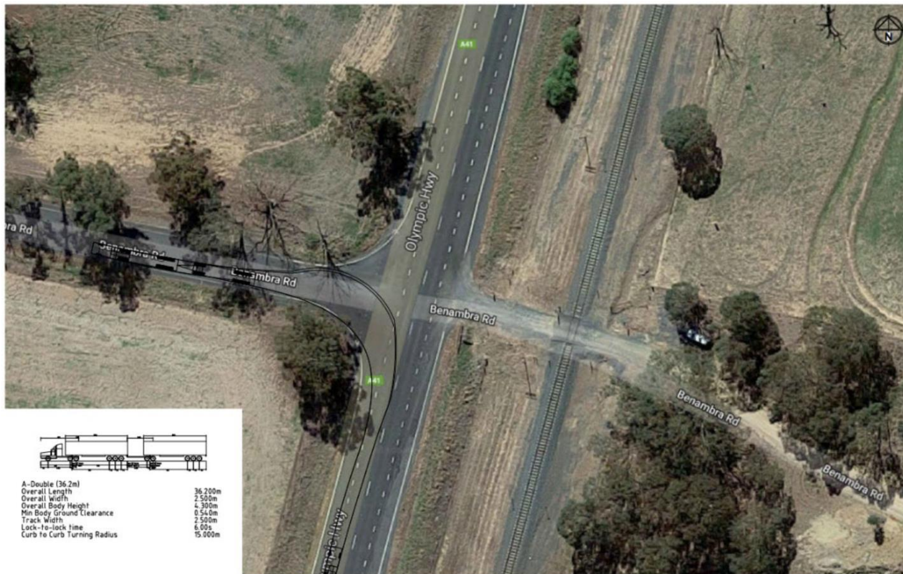
Figure 3-15 Swept path analysis turning left into Benambra Road
