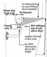
Ensure handrails are installed at a consistent height between 865-1000mm height above step nosing or FFL ramp surface, compliant with AS1428.1 Clause 12d.
