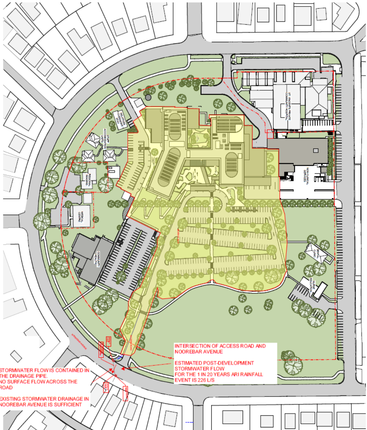
Figure 6: Stormwater Drainage Catchment and Estimated Stormwater Flows Post-Development
