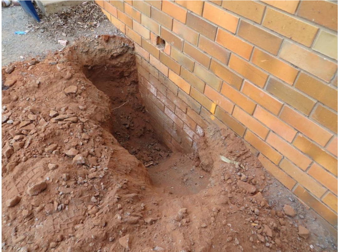
Photo 14. View of test pit (TP121) excavated adjacent to General and Medical Ward Building
