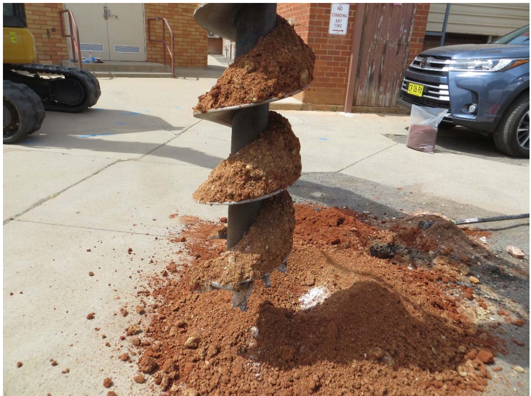
Photo 6. Soil and weathered rock profile encountered in BH103 in vicinity of Staff Dining Room and Kitchen
