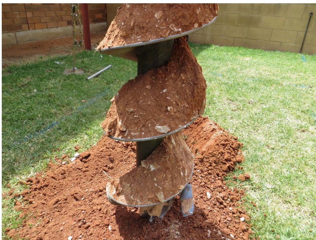
Photo 8. Soil and weathered rock profile encountered in BH113 in vicinity of Oncology and Specialist Clinic 1
