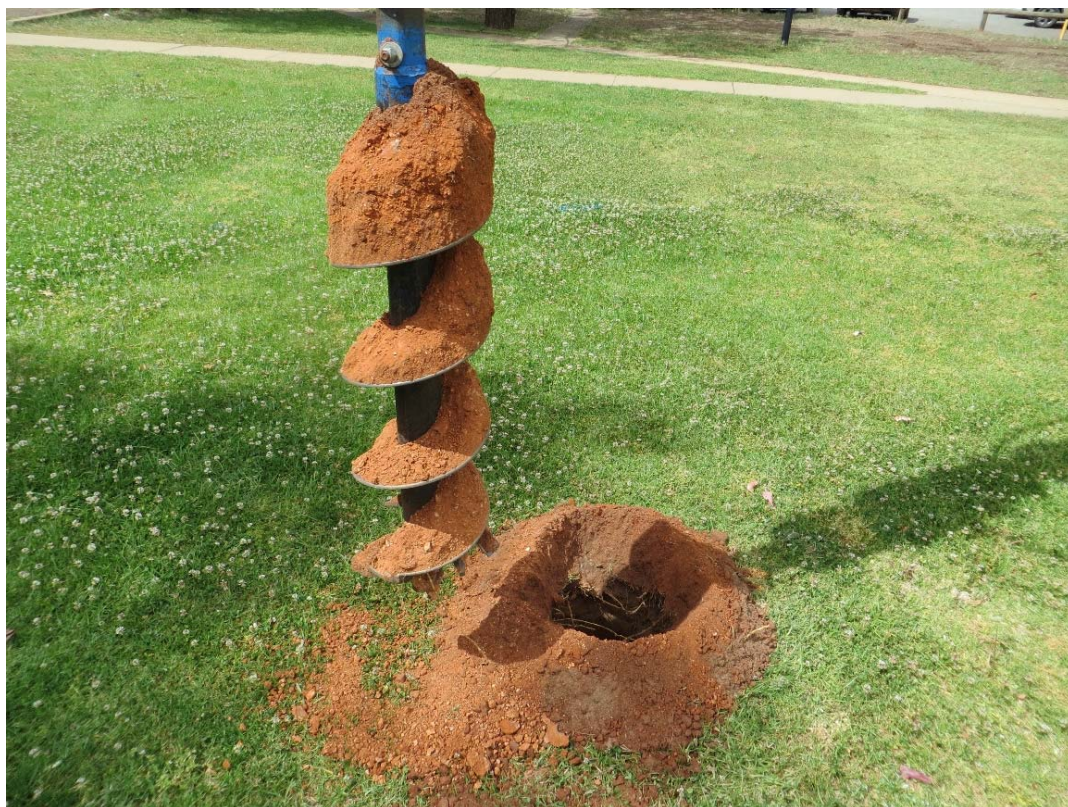
Photo 7. Soil and weathered rock profile encountered in BH111 in vicinity of Nurses Training School
