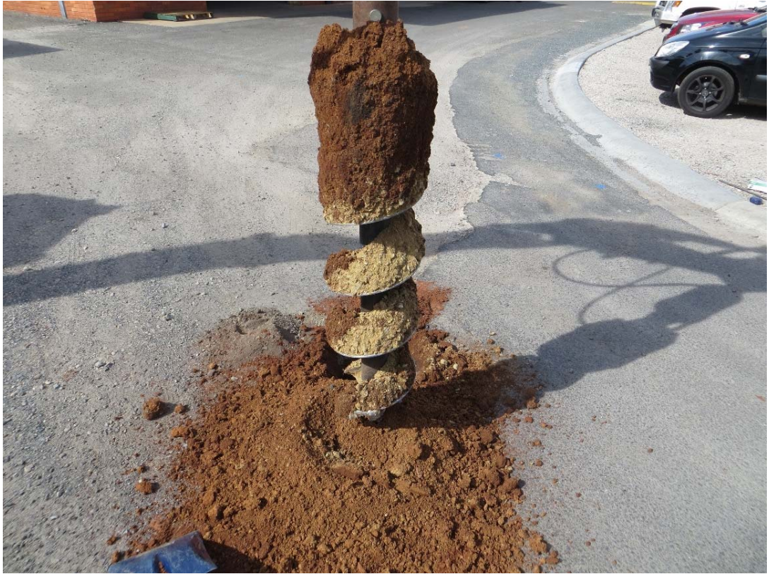
Photo 5. Soil and weathered rock profile encountered in BH100 in vicinity of Bulk Workshop
