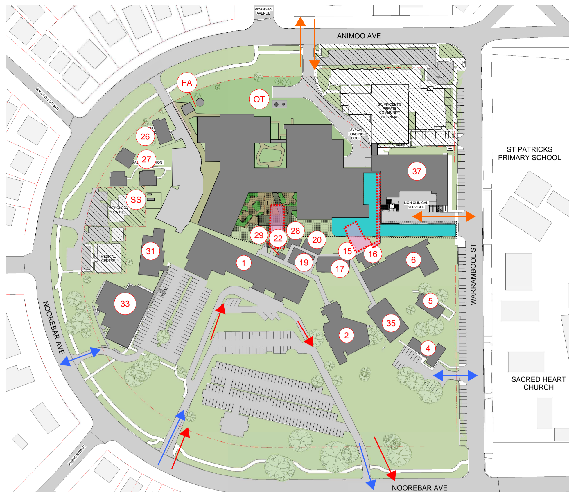
STAGE 2 (Q3 2024 to Q4 2024) Demolition of buildings 15 & 22 and construction of southern courtyard and ambulance entry.
