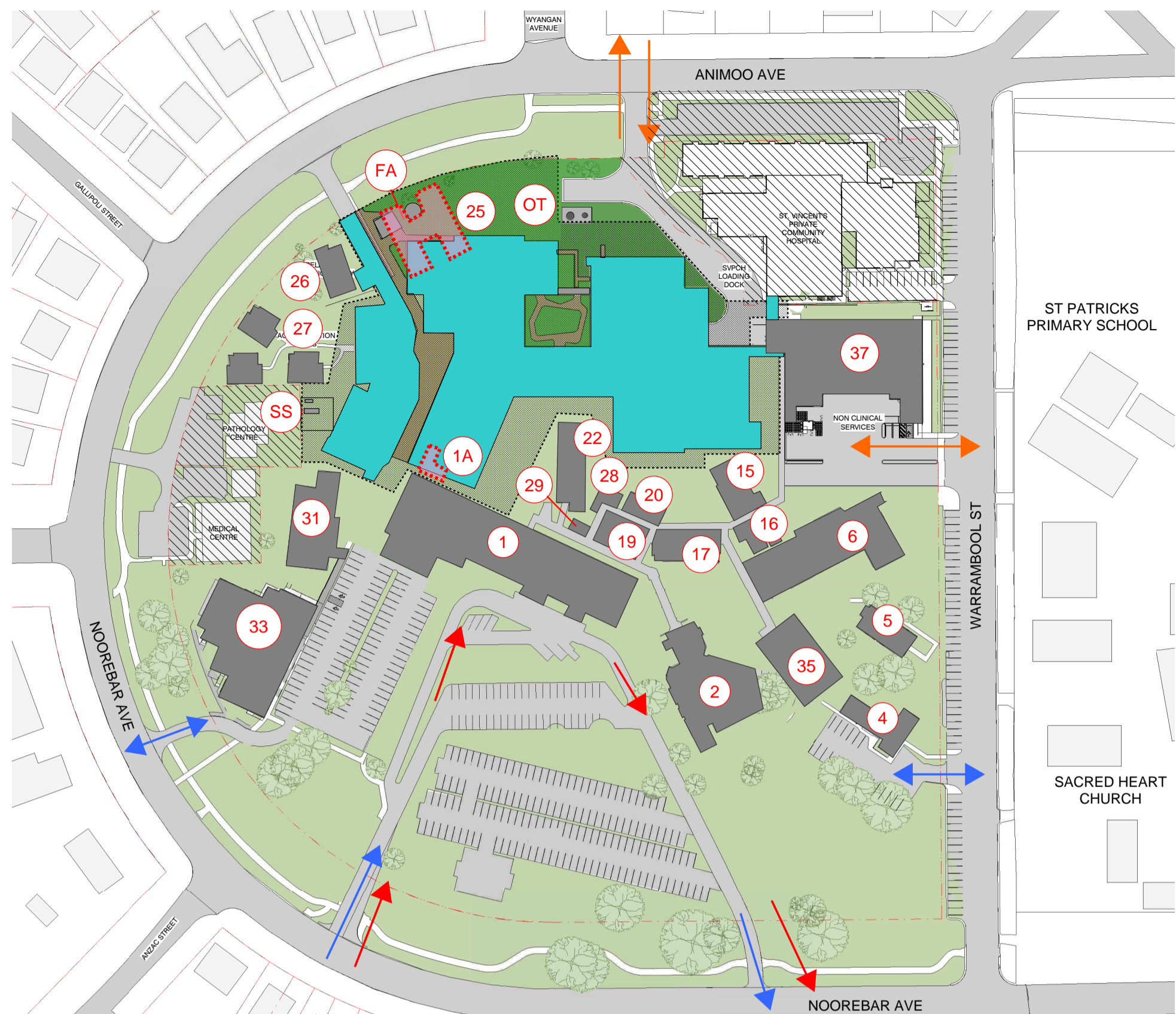
STAGE 1 (Q1 2022 to Q3 2024) Demolition of Building 25 & relocation of mechanical plant within Main Works Boundary. Installation of new site infrastructure (substation / generator / fire system). Construction of new Clinical Services Building, linkages to NCS & SVPCH & western carpark, northern landscape works.
