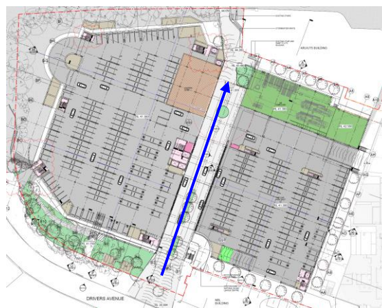
Figure 14: Carpark Level 0 (pressure driven flow indicated by blue line)
