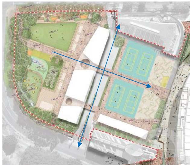
Figure 13: Walkways alignment to prevailing wind directions (blue lines)
