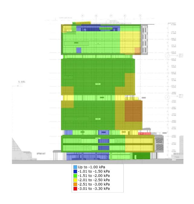
Figure 2a: Negative Peak 1000 year return period Ultimate Net Pressure Zone Diagram – North Elevation
