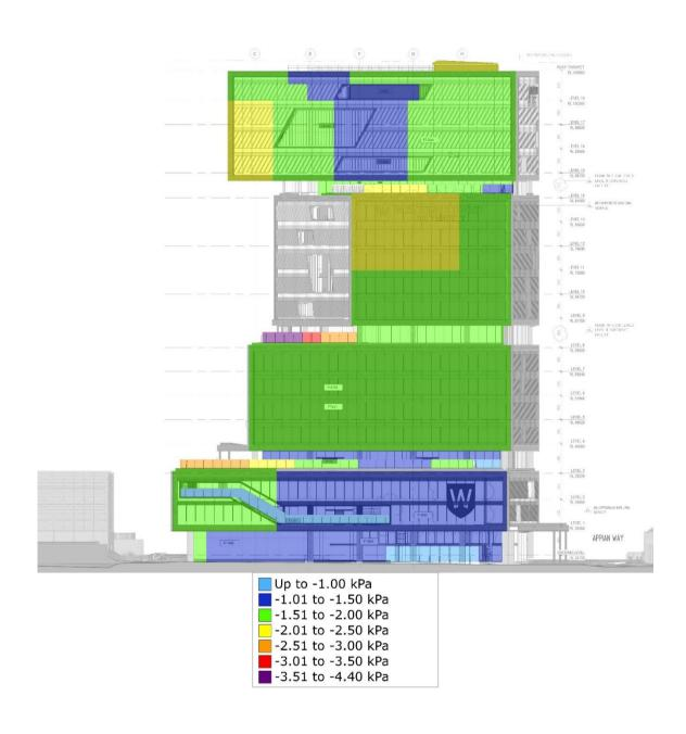
Figure 2c: Negative Peak 1000 year return period Ultimate Net Pressure Zone Diagram – South Elevation
