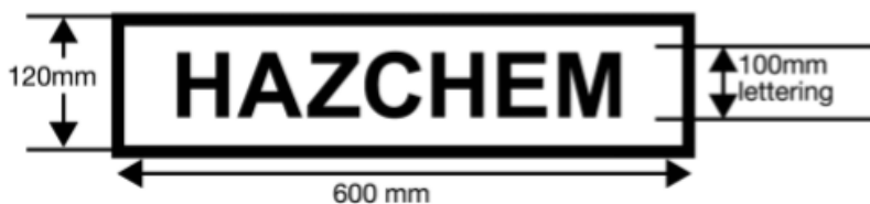
Figure 5. Form and dimensions of outer warning placard.
