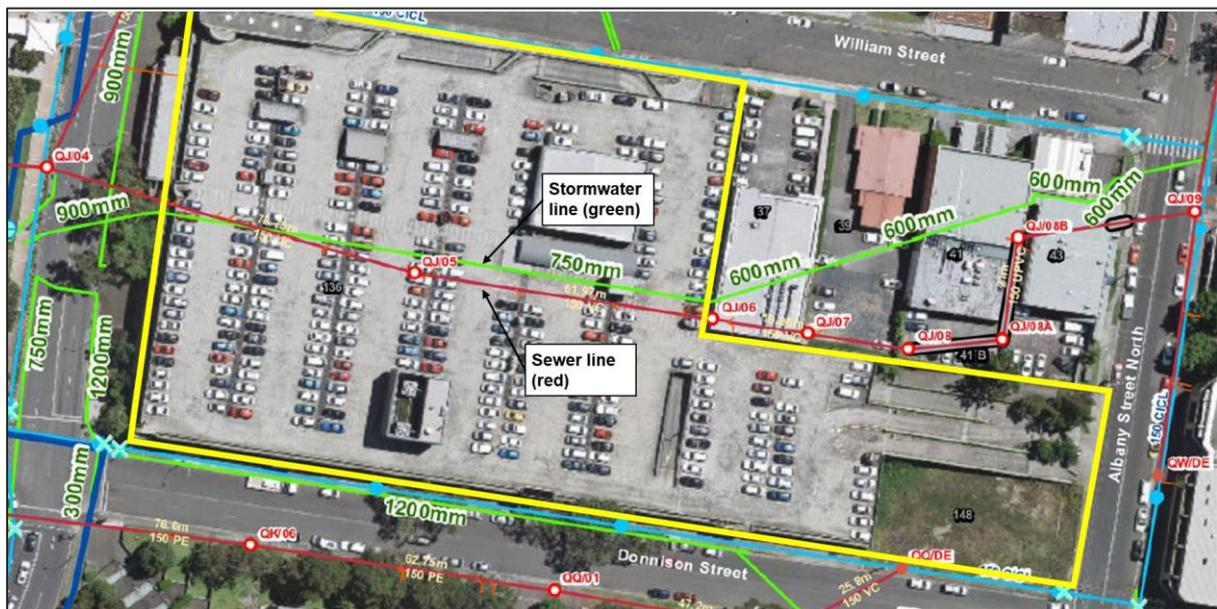
**Figure 26** | Location of stormwater (green) and sewer (red) pipes crossing the site (yellow) (Base source: Applicant's EIS)
