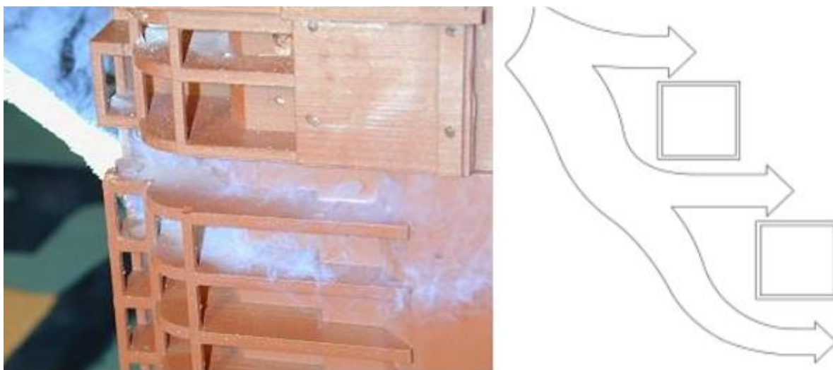
Figure 10: Visualisation through corner balconies (L) and channelling between buildings (R).
