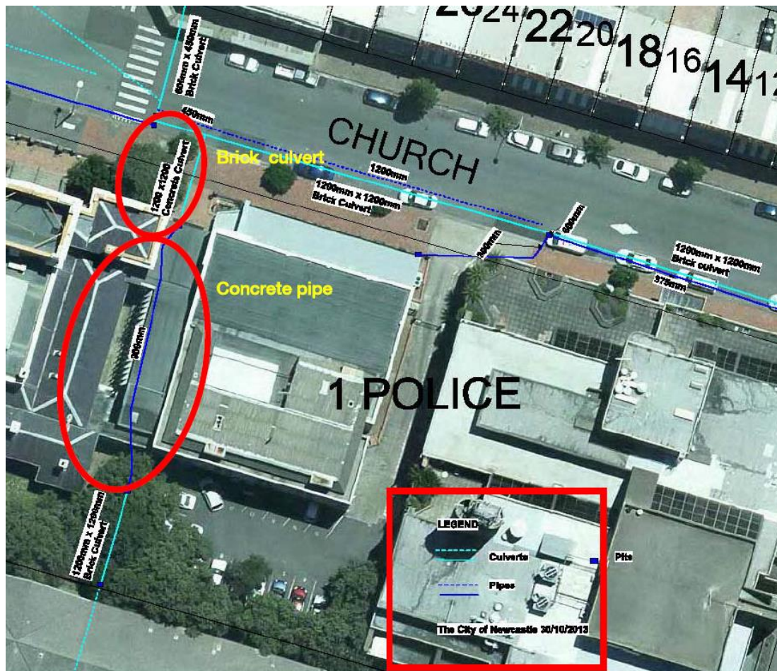
Figure 3.6 Plan reproduced from the CMP, showing location of post-1861 culvert and perceived brick-lined (light blue) and concrete pipe portion (dark blue) beneath administration building.
