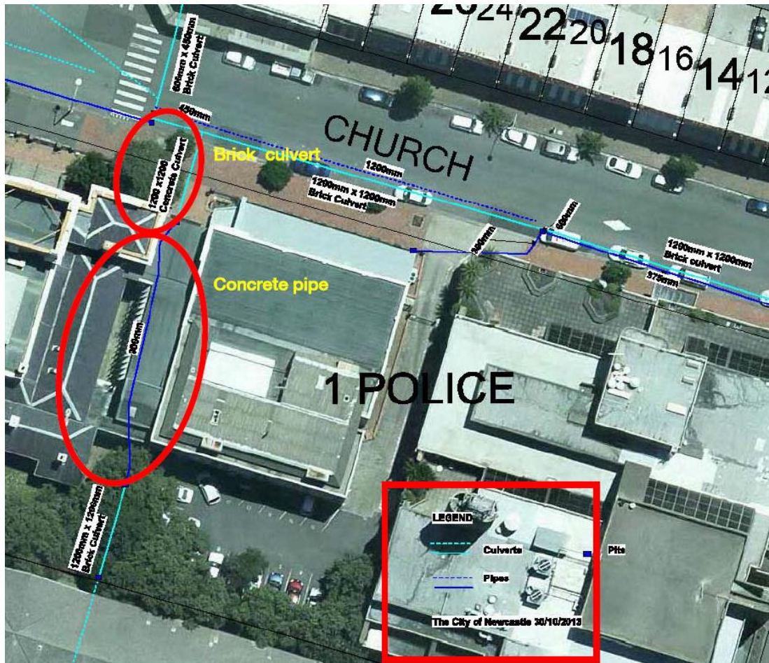
Figure 3.13 Plan reproduced from the CMP, showing location of post-1861 culvert and perceived brick-lined (light blue) and concrete pipe portion beneath administration building.
