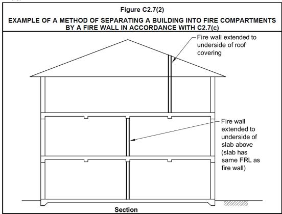
For a fire wall to compartment a building it must extend to the underside of any roof covering or between floors that have an equivalent FRL to the fire wall.
