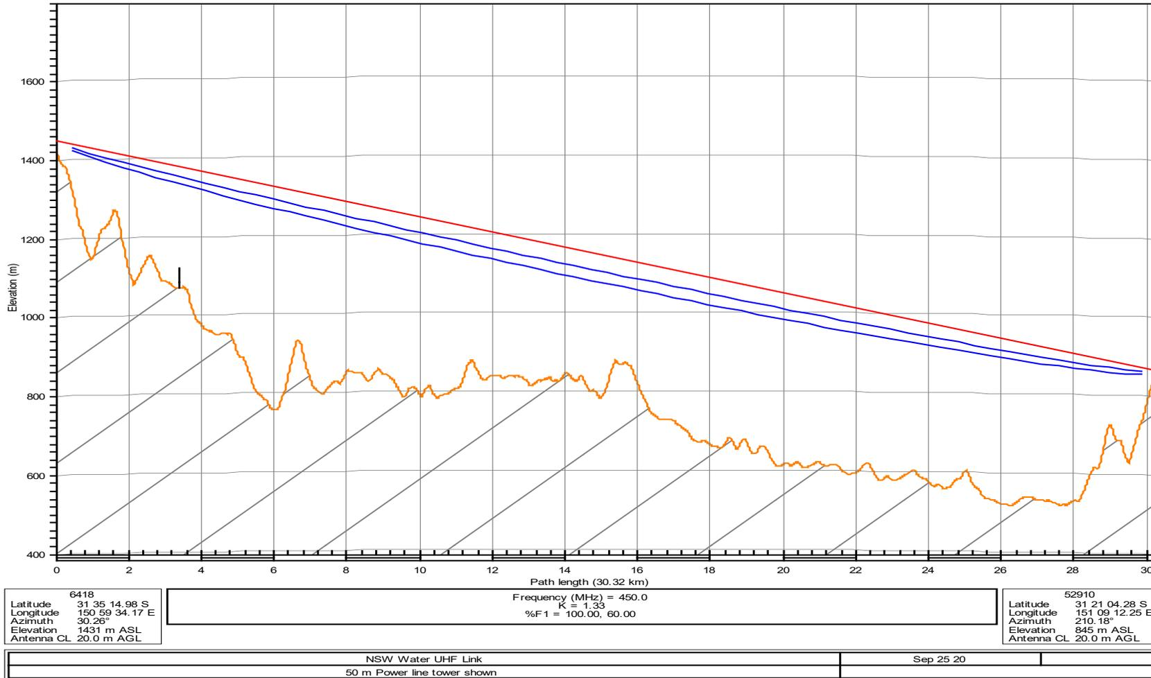
ATTACHMENT 14 – SES LINK VERTICAL PATH PROFILE SHOWING POWER LINE CLEARANCE
