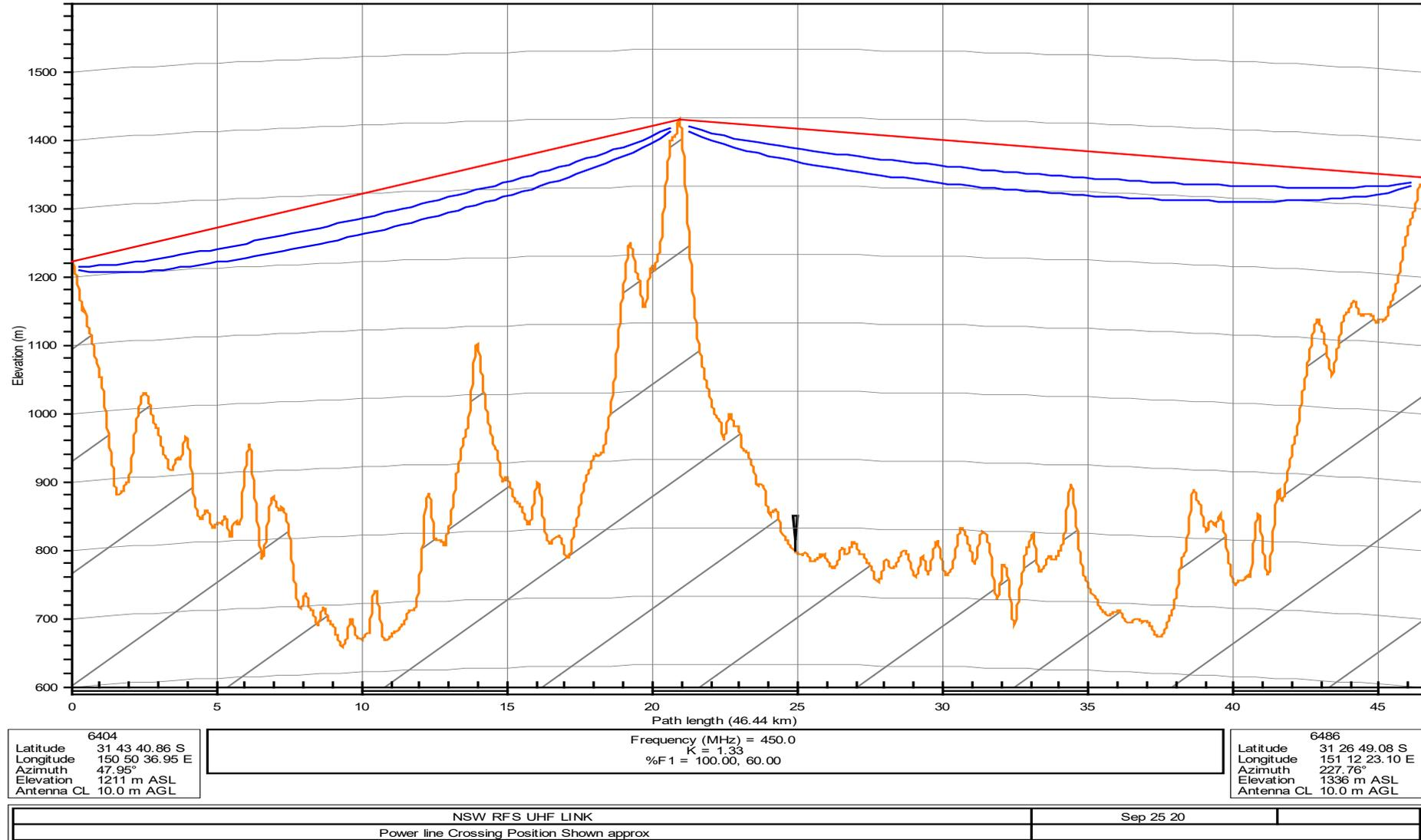
ATTACHMENT 12 – NSW GOVT TELCO LINK VERTICAL PATH PROFILE SHOWING POWER LINE CLEARANCE
