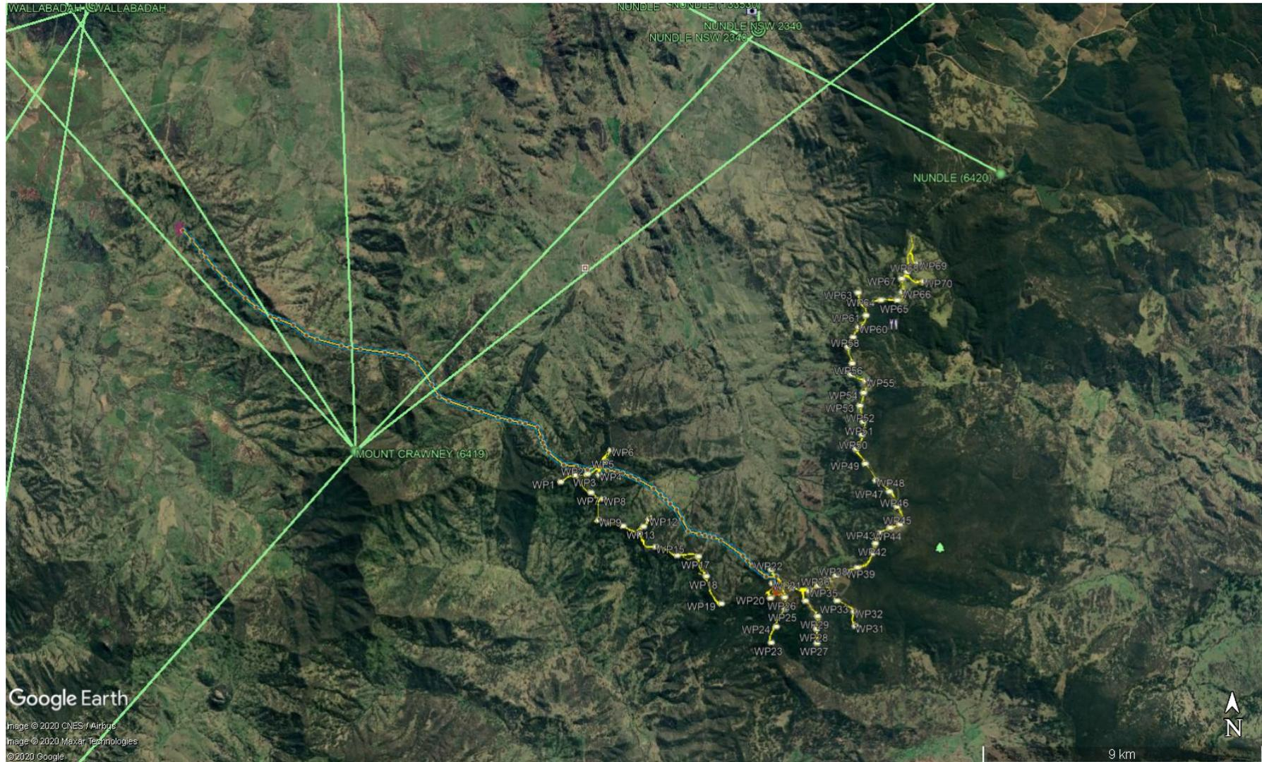
ATTACHMENT 6 VHF TELSTRA RADIO LINK PATHS NEAR WIND TURBINES
